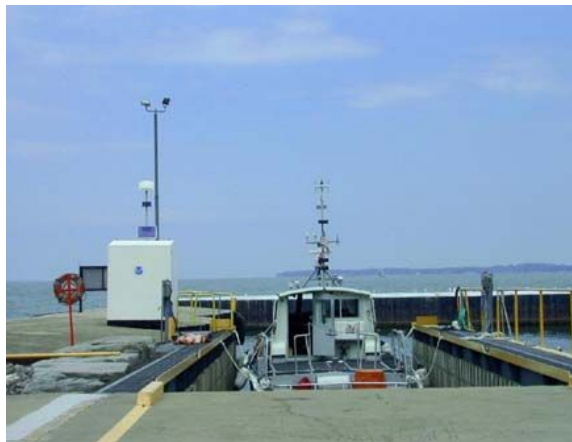
Figure 4.11. The Marblehead water level gauge located in the Marblehead Coast Guard Base. The white box to the left of the boat is the gauge house built by CO-OPS.
