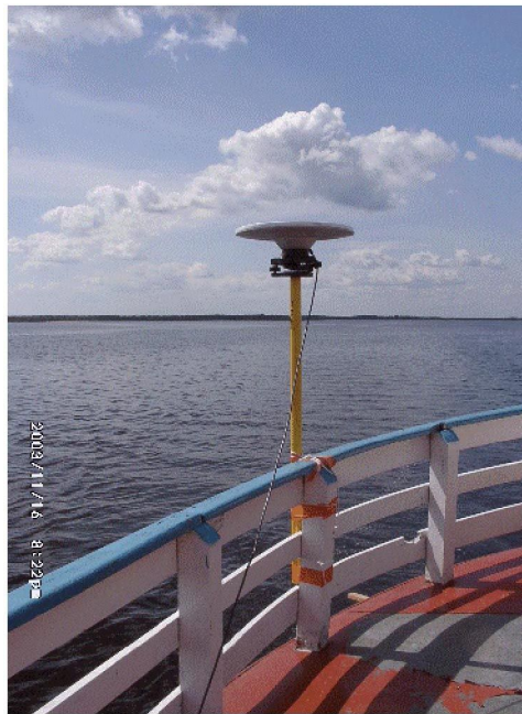
Figure 5.2. The GPS ship (top left), the GPS buoy (top right), and the on-board GPS antenna (bottom), used in the campaign (Insitute de Recherche pour le Développement, 2003).
