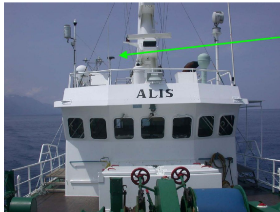
Figure 4.16. The main GPS antenna on the roof of the vessel ALIS (Courtesy of V. Ballu).
