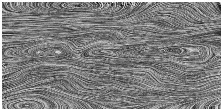
Figure 4.6: LIC image of the 573x288 ocean wind dataset in 1.9s, using convolution length 30.
