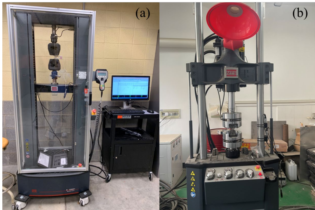
Figure A-15. Tensile testing machine: (a) MTS E44 universal testing machine, and (b) MTS LandMark 370 universal testing machine.
