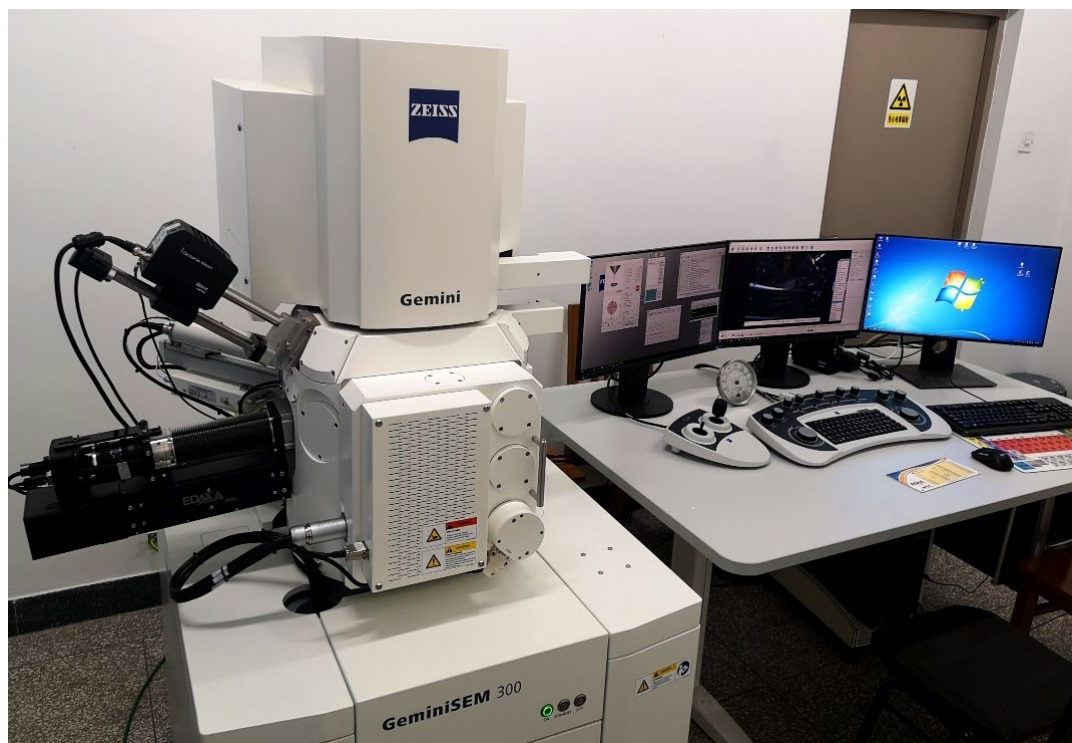
Figure A-9. FESEM (Carl Zeiss Ultra Plus, Carl Zeiss, Oberkochen, Germany)
