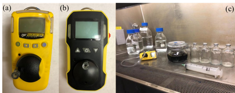
Figure A-7. (a) H 2 S sensor, (b) H 2 sensor, and (c) gas dilution syringe and bottles.
