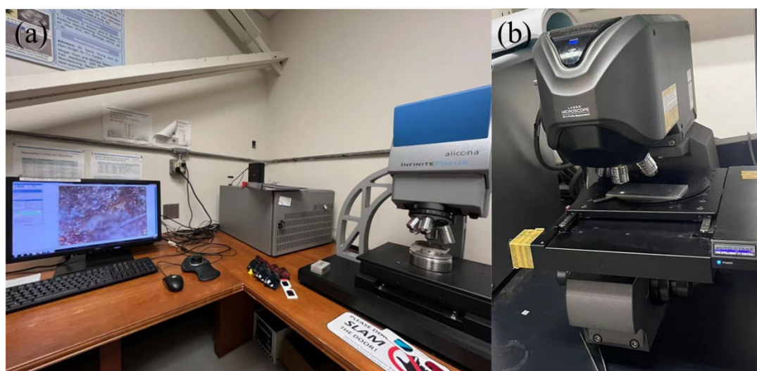
Figure A-12. IFM Model ALC13 machine (a), and CLSM VK-X250K machine (b).
