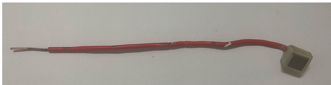
Figure A-2. Image of working electrode set up using X80 square coupon.
