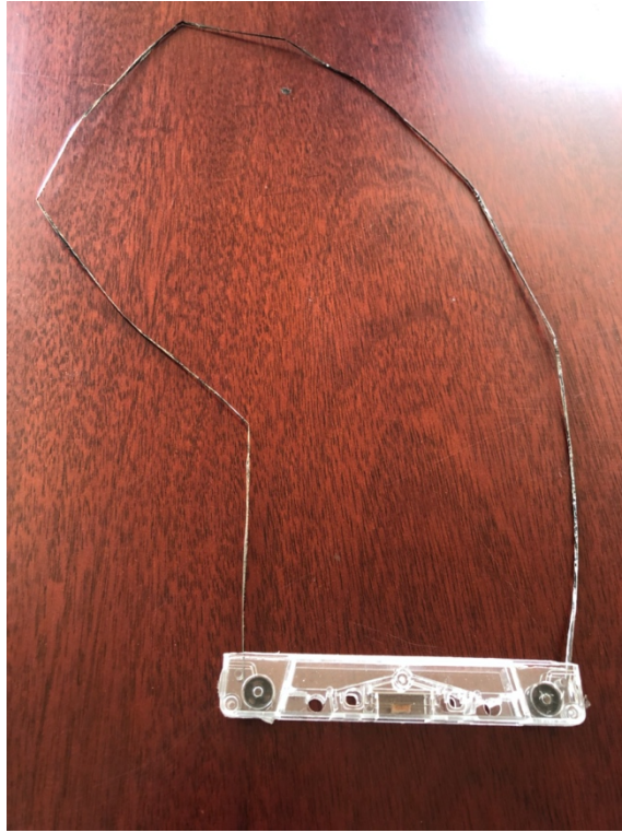
Figure 32. Original tape loop with damage.
