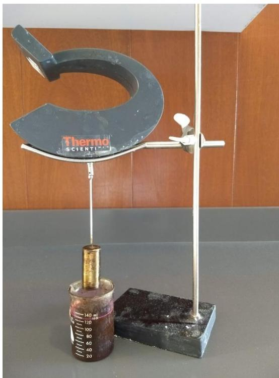
Figure 7. Setup used for viscosity testing, showing Thermo Scientific viscotester and one of the 140 mL containers used for all samples.
