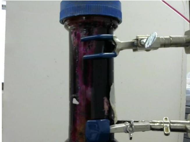
Figure 9. Vertical column used in dry sand column test.
