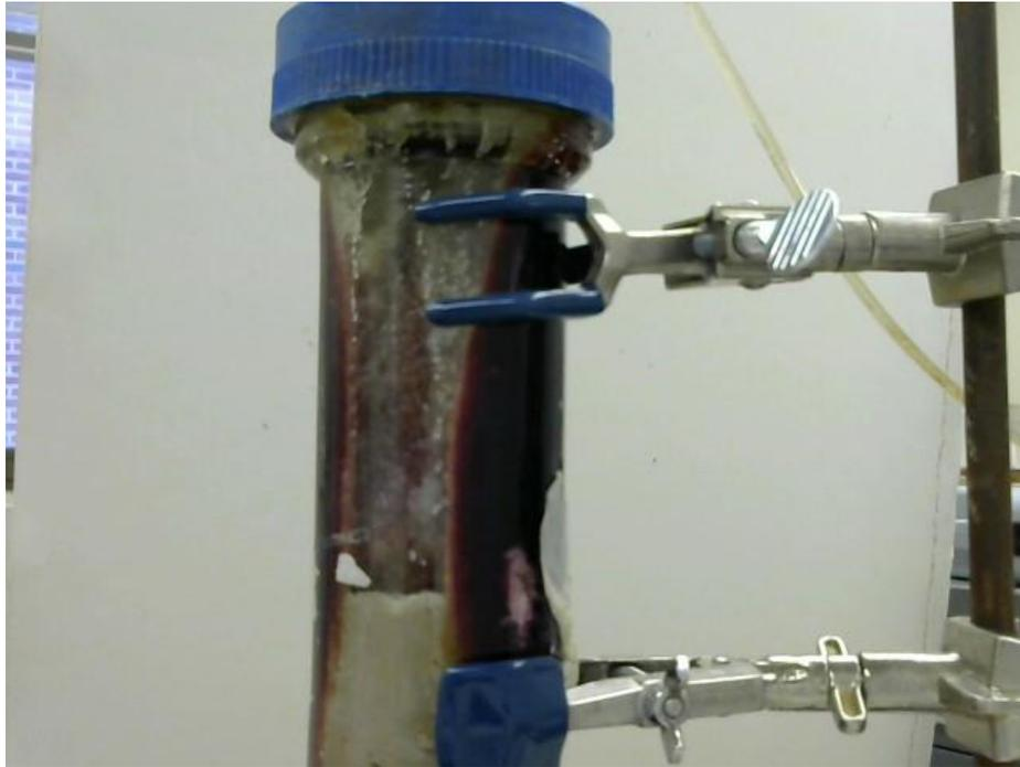
Figure 18. The open channel where water was pumped through the column. Areas where permanganate has been depleted are clearly marked by the presence of white sand. Unseen at the top of the column is solid layer of glassy gel indicative of the solidity obtained after gelation in the absence of water.
