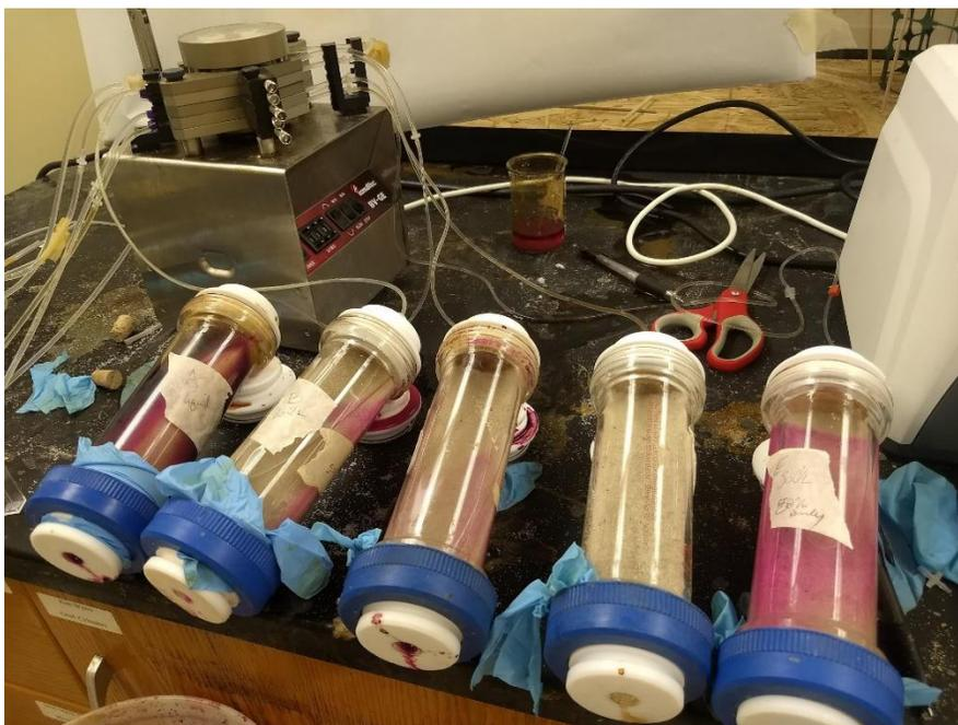
Figure 8. Experimental setup for the second round of column testing. Ismatec peristaltic pump is visible on the left, pumping water through five columns, one of which failed to give usable data. Latex around the edge of the bottom cap ensured a watertight seal.
