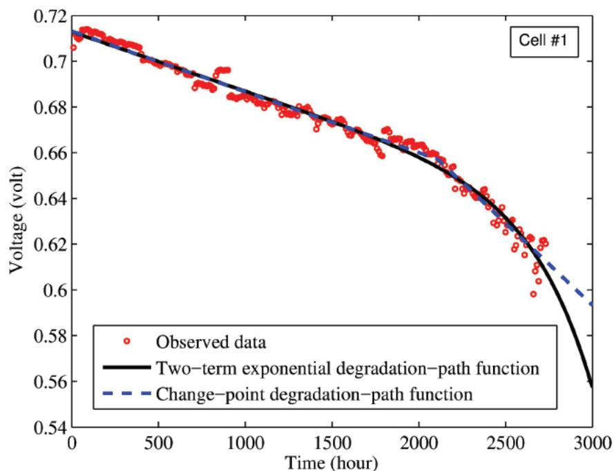
Figure 9. Comparison between the two degradation modeling fits\_Posterior medians of two degradation models fitted to the degradation data of fuel stack cell #1
