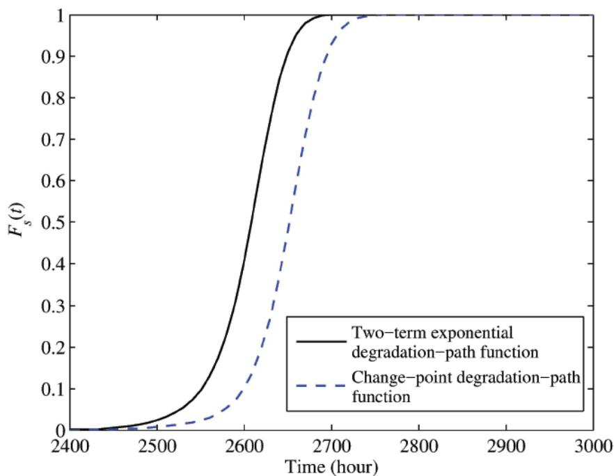
Figure 10. Comparison between the two degradation modeling fits\_Posterior medians of the stack failure-time distribution  $F_s(t)$  when  $k = 1$
