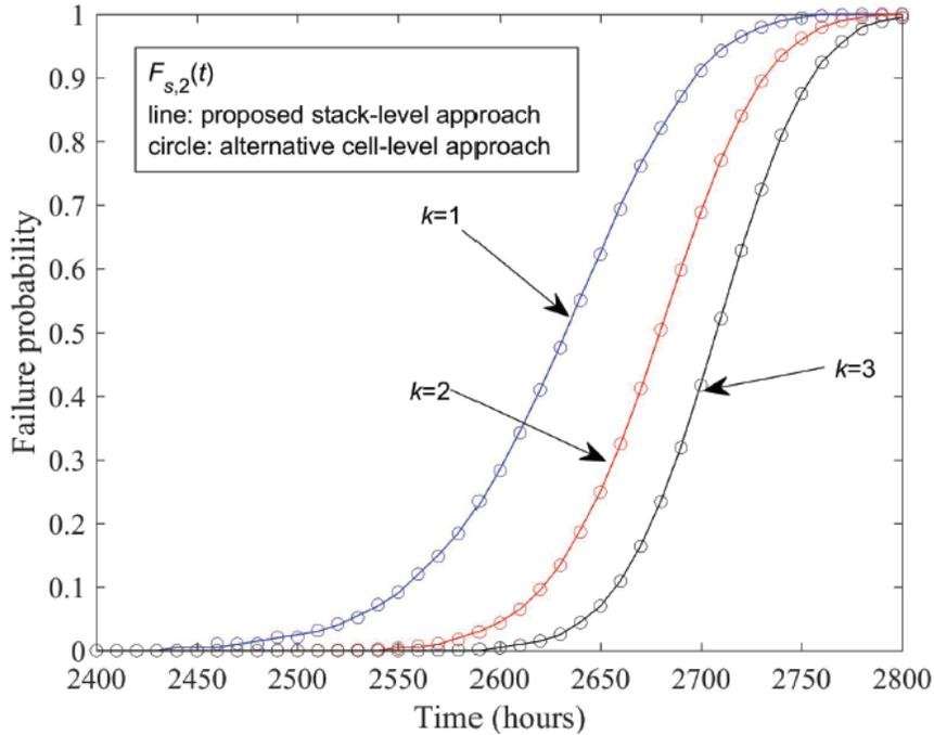
Figure 7. Posterior medians of the failure-time distributions for a randomly selected stack using two different approaches by considering the minimum cell voltage measure only
