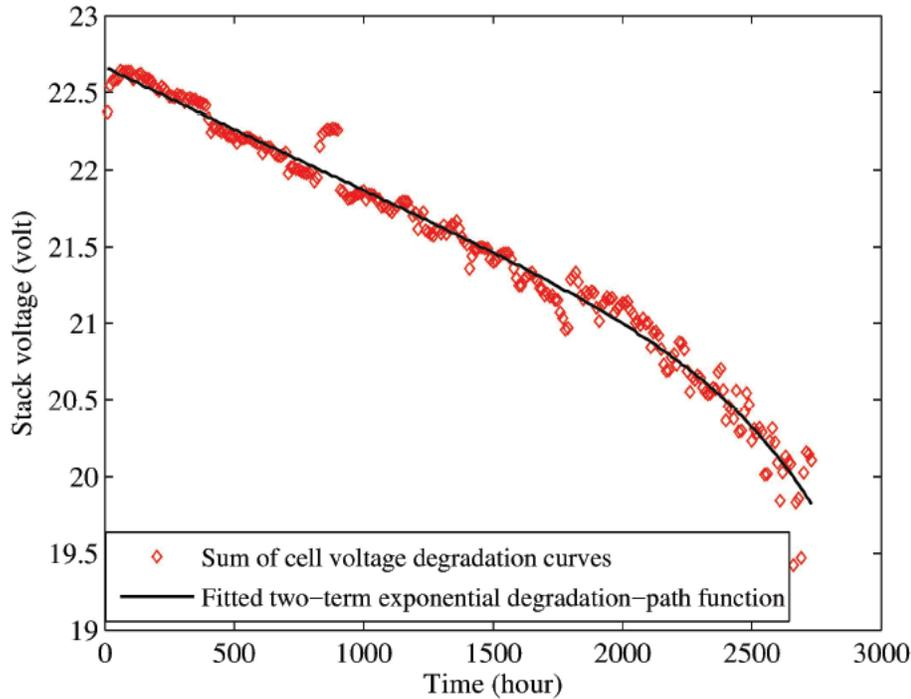
Figure 8. The stack output voltage degradation curve obtained by summing individual degradation levels of cell voltage and the fitted two-term exponential degradation-path function
