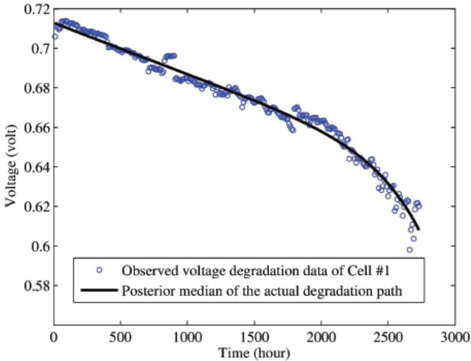
Figure 3. Posterior median fit to the degradation-path for fuel cell #1
