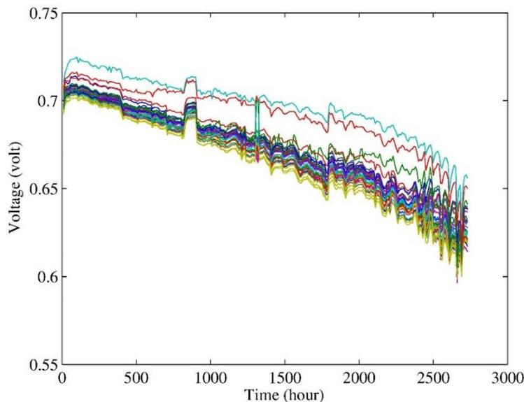
Figure 2. Observed voltage degradation-paths of 32 fuel cells in a tested PEMFC stack system [3]
