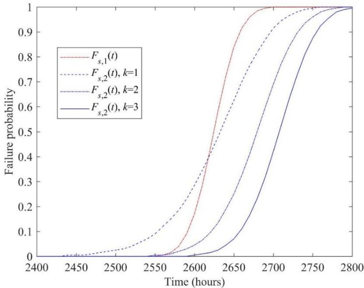
Figure 4. Posterior median estimation of  $F_{s,1}(t)$ , and  $F_{s,2}(t)$  for  $k = 1, 2, 3$
