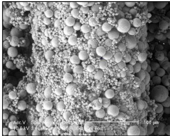
Figure 3.3: SEM image of line formed by bimodal powder of 20 \mu\text{m} spherical and 5 \mu\text{m} equiaxial alumina powder (12.5 wt%) [80].
