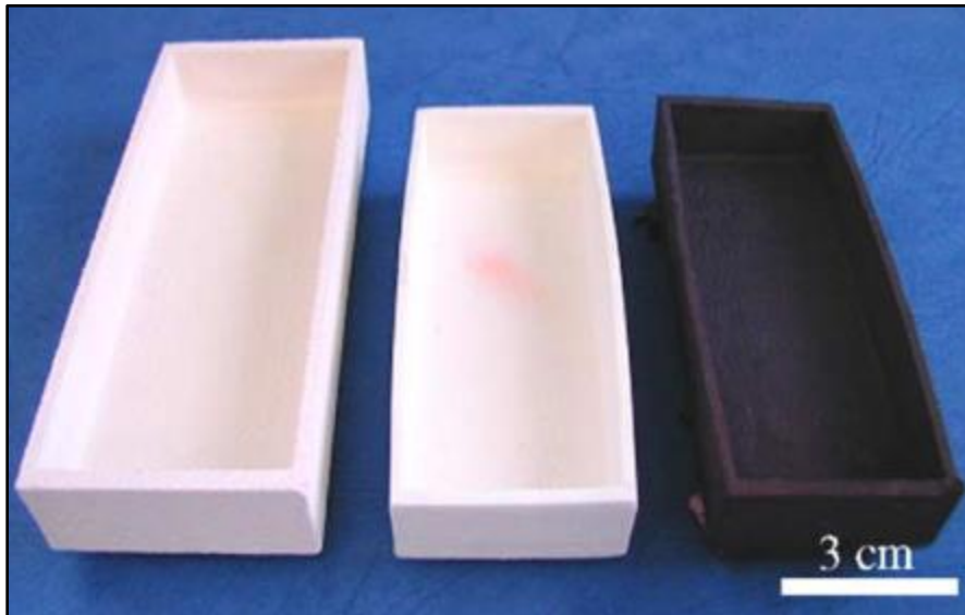
Figure 3.2: Printed green part of alumina (left), sintered alumina part (middle) and copper infiltrated alumina part (right) [77].
