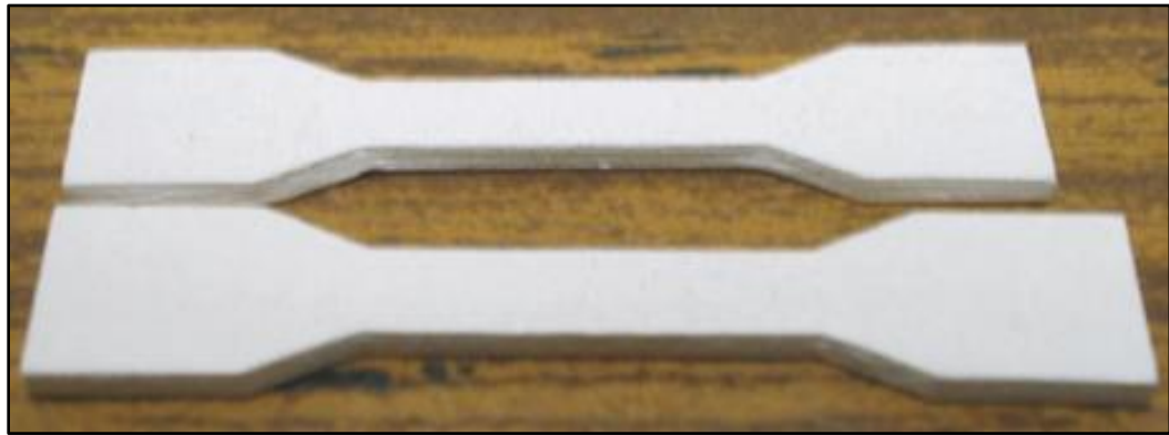
Figure 3.4: Substantial difference in the shrinkage of the sintered parts printed without (top) and with nanoparticles (bottom) [52].
