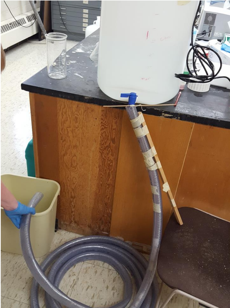
Figure 3-3: Flow through test setup during test with forms in place and tied to wooden skewer. Enough twine was left at the top of the string of ten forms, so that once in place, the forms would sit below the head of the outflow.
