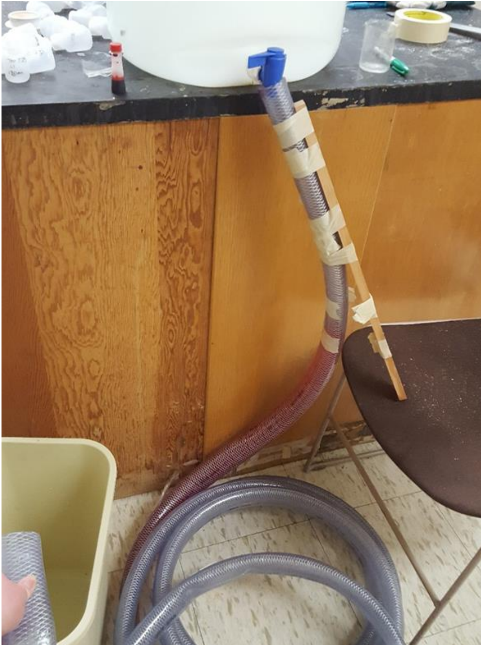
Figure 3-5: Dye test conducted using red food coloring. Dry to outflow test was conducted first. Once outflow began dye was added.
