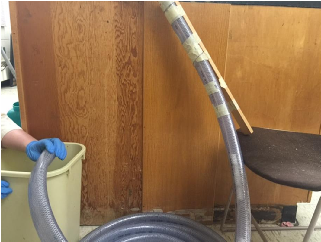
Figure 3-4: Flow through test set up. PVC tubing loaded with ten forms.
