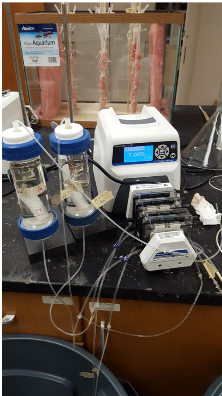
Figure 3-2: Smaller size of HP SR forms used in release rate test. These two were part of a suite of 12. The flow-through test utilizes the other 10.
