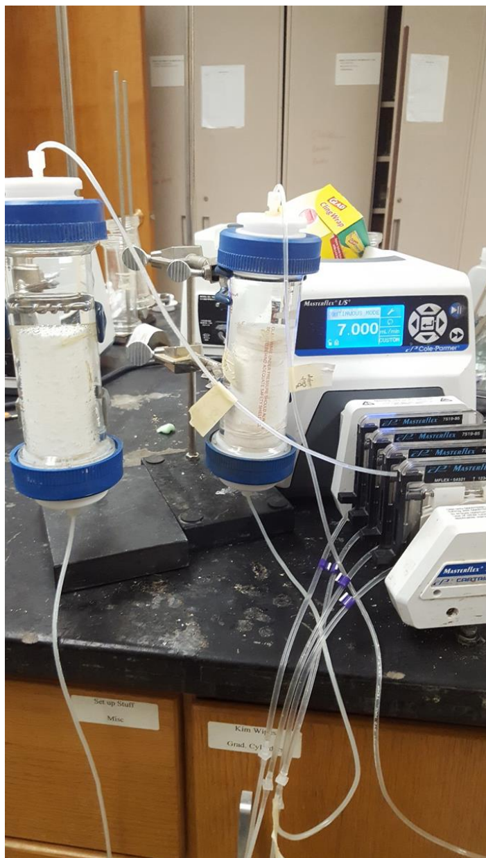
Figure 3-1: Larger size of form used in release rate test in columns connected to Masterflex set at 7ml/min.
