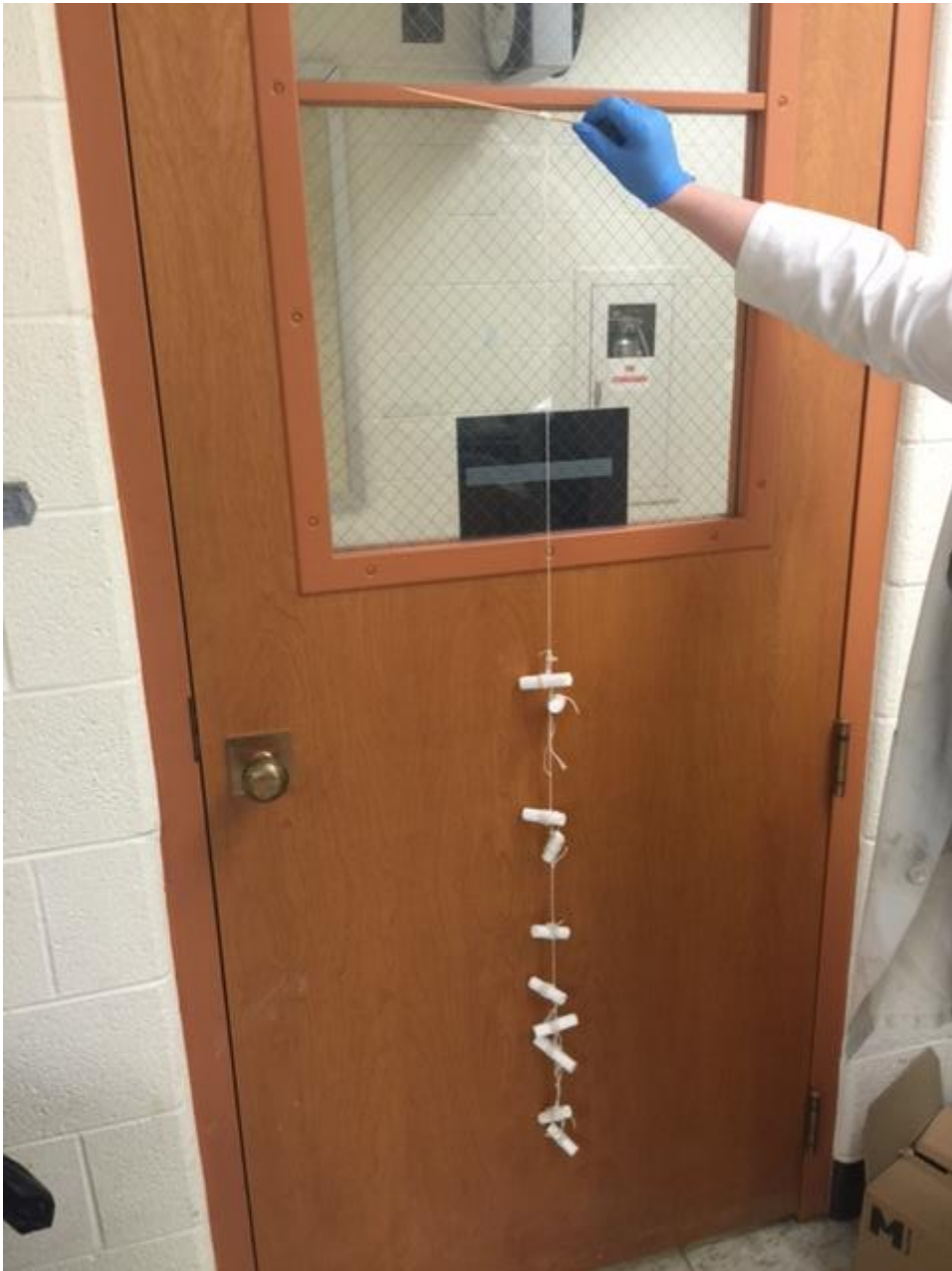
Figure 3-6: String of the ten SR-HP forms tied together with cotton twine used in flow-through test.
