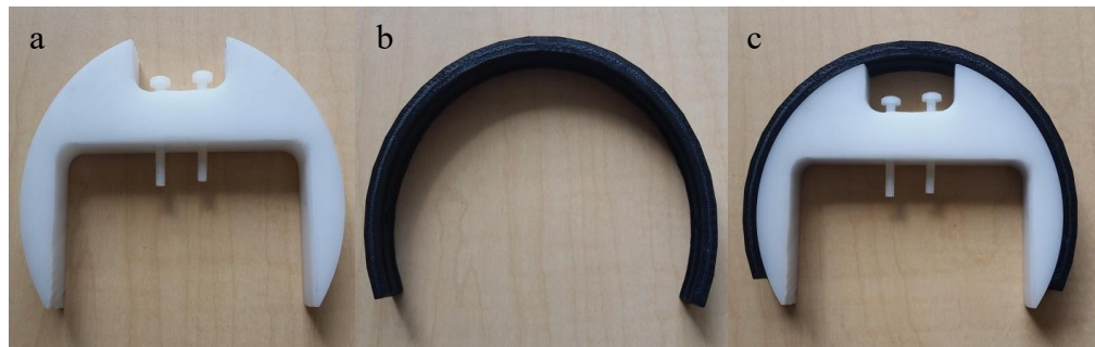
Figure 16: Clamp assembly: (a) Inner clamp, (b) Outer clamp, (c) Inner-Outer clamp assembled.
