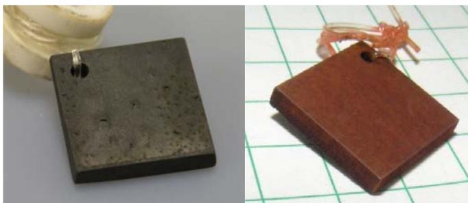
Figure 88. Steel samples after 2 days of immersion without (left) and with O<sub>2</sub> (right).
