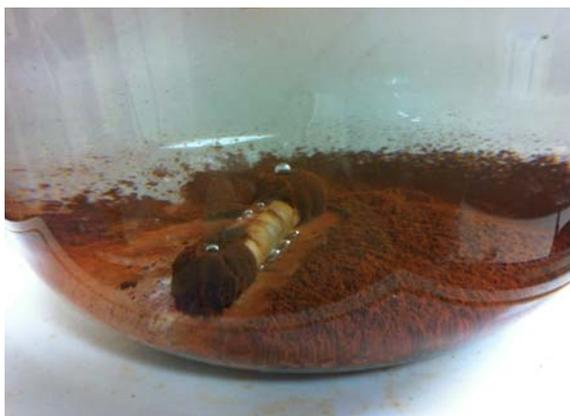
Figure 35. Reddish brown precipitate at the bottom of the glass cell.
