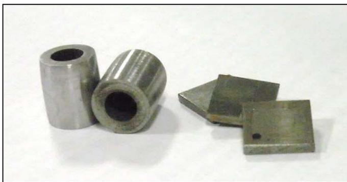
Figure 9. Steel specimens for glass cell tests
