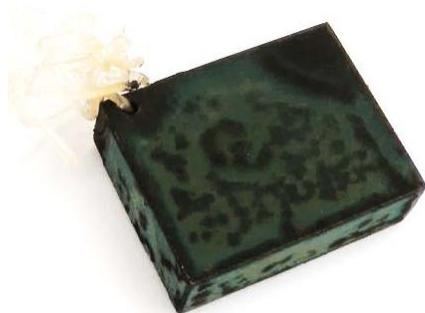
Figure 65. Bluish-green corrosion product on a recovered steel specimen for experiment at 25°C, 40 bar pCO<sub>2</sub>, with 4% O<sub>2</sub>
