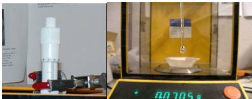
Figure 12 Weight drop method for determining the surface tension.
