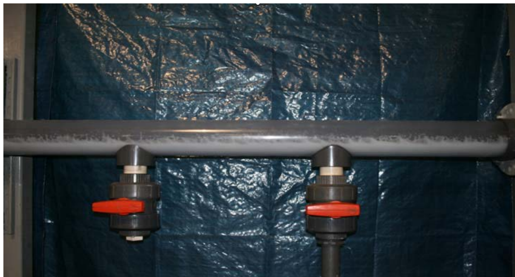
Figure 80. Formation of foam in the Hilly-Terrain system when the flow loop has 20 ppm of inhibitor P1.
