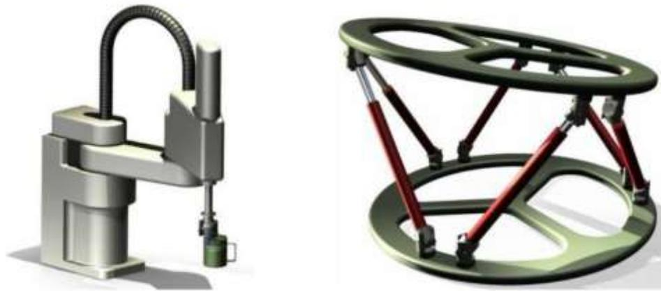
Figure 1: Serial and parallel robot
