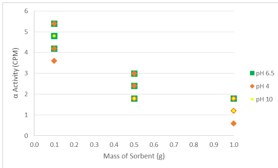
Figure 5-15: Additional Solution 3 Batch Tests to Evaluate pH Variation Using Powdered Clinoptilolite
