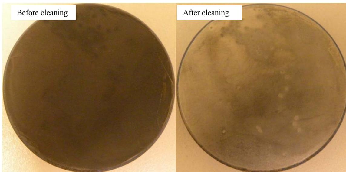
Figure 6.52 View of the experiment specimen #2 after 14 days exposure at test condition: 25°C, pH 5, 1 wt% NaCl solution saturated with CO<sub>2</sub>.
