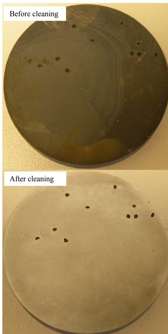
Figure 6.19 View of the experiment sample #1 after 25 days exposure with corrosion product layers and without corrosion product layers at test conditions 25°C, pH 5, 1 wt% NaCl solution saturated with CO<sub>2</sub>.
