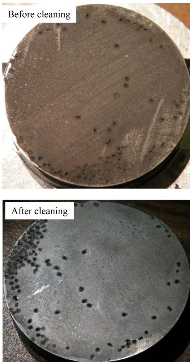
Figure 6.10 View of the steel surface showing a lot of pits after 40 days exposure at conditions 25°C, pH 5, 1 wt% NaCl solution saturated with CO<sub>2</sub>.
