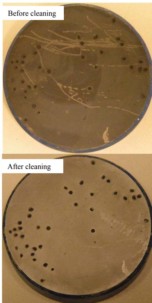
Figure 6.24 Views of the experiment sample #2 after 34 days exposure with corrosion product layers (left) and without corrosion product layers (right) at test conditions 25°C, pH 5, 1 wt% NaCl solution saturated with CO<sub>2</sub>.
