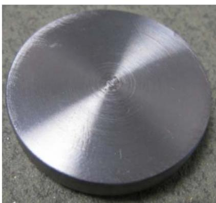
Figure 4.2 View of an API 5L X65 mild steel experiment specimen.
