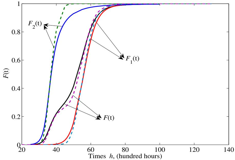
Figure 4.4:  $F(t)$  comparison with two components in GaAs laser model
