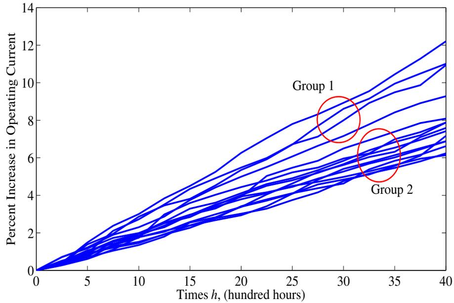
Figure 4.2: Plot of percent increase in operating current for GaAs lasers tested at 80°C with 2 subgroups
