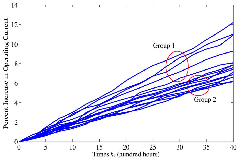
Figure 4.1: Plot of percent increase in operating current for GaAs lasers tested at 80°C
