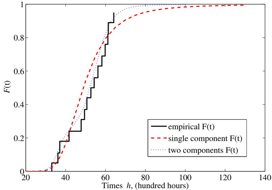
Figure 4.8: Comparison among probability plot,  $F(t)$  with single component and two components in GaAs laser model
