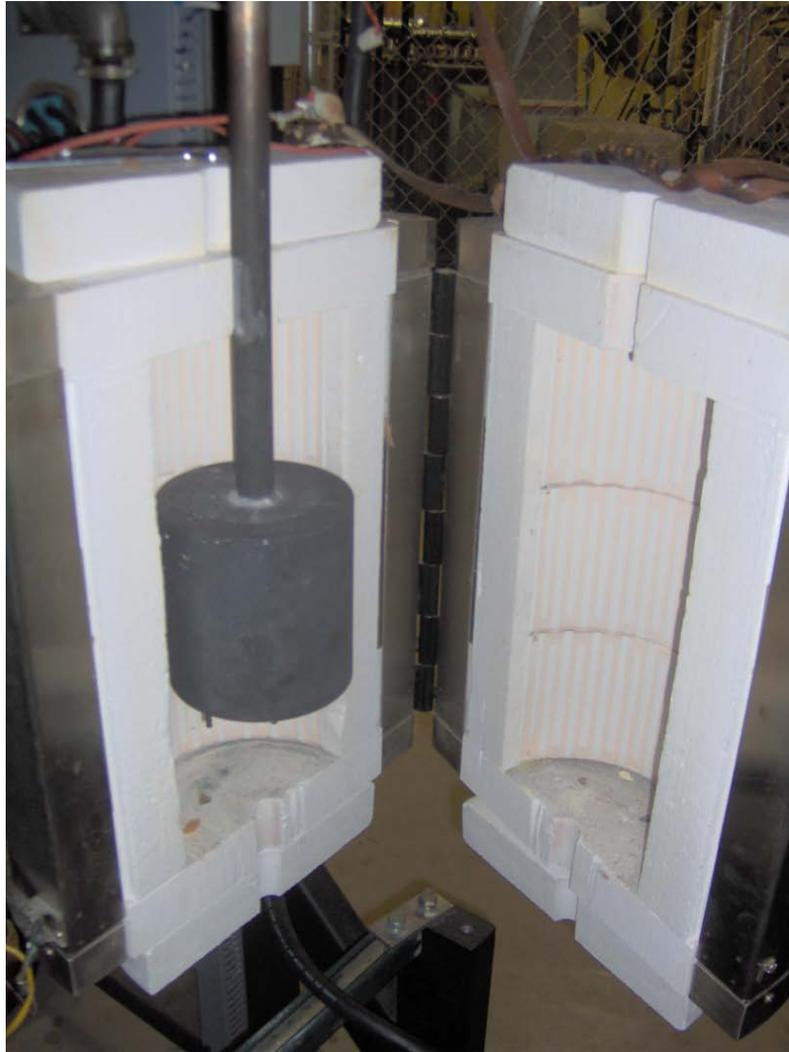
**Figure 3.2 Can arrangement in test stand furnace**
