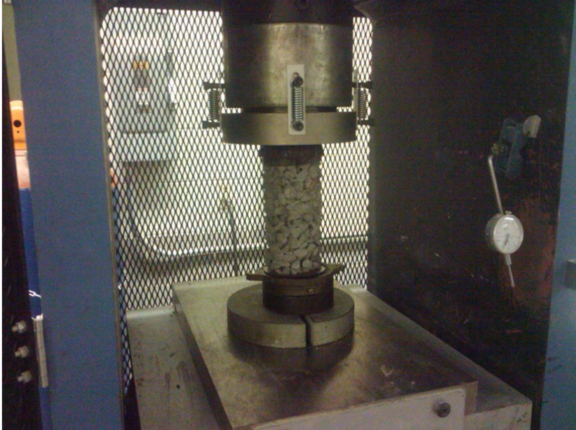
Figure 3-4. Concrete specimen under the test
