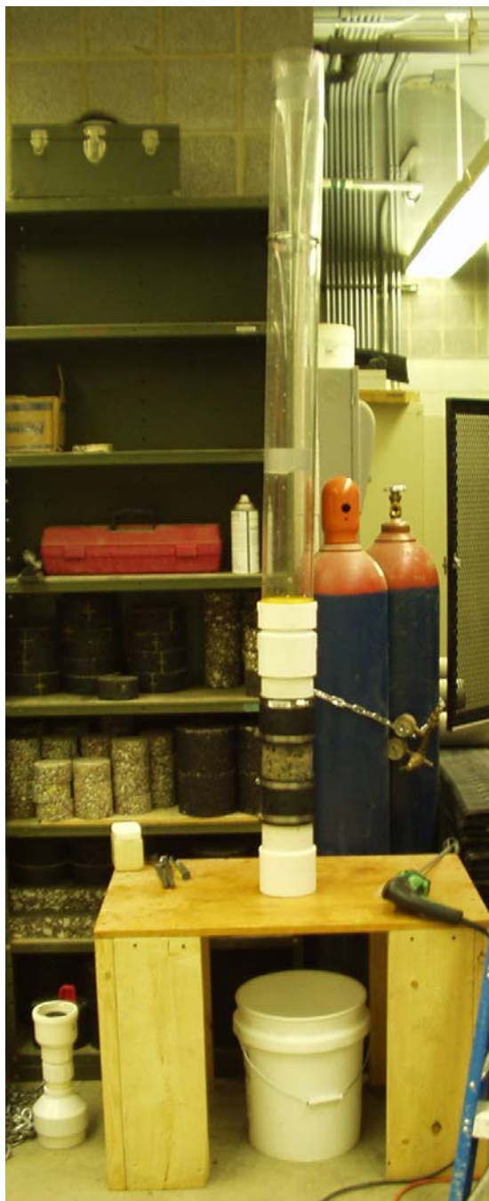
Figure 30-3. Vertical I-shaped permeameter with core mounted
