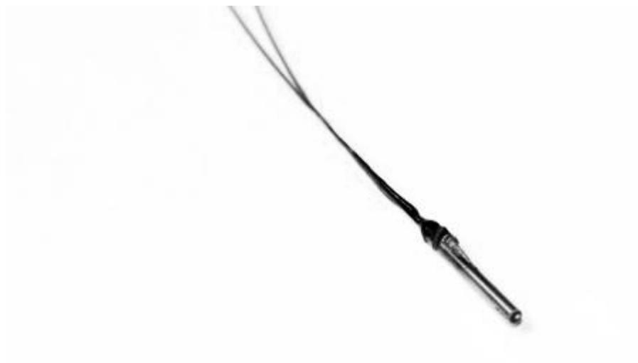
*Figure 66.* One conductivity probe, 160 conductivity probes are used in the doughnut cell.
