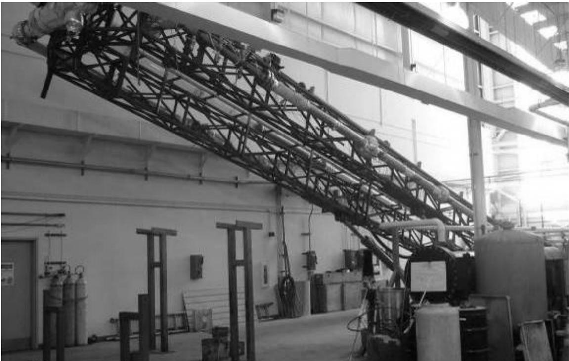
*Figure 69.* Picture of the flow loop in 15° position.
