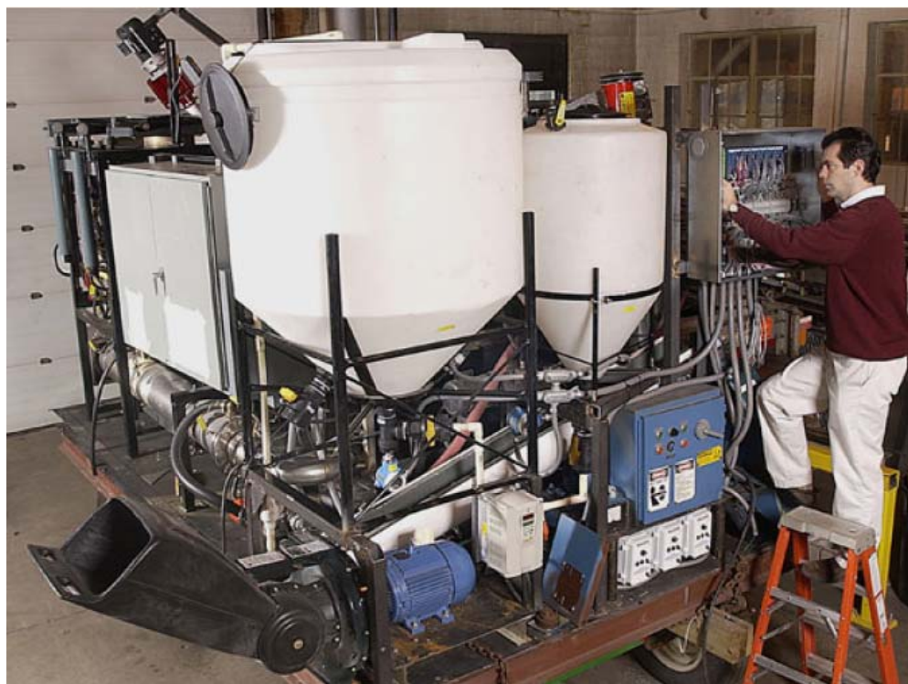
Figure 6. Tactical/mobile refinery design and refinery under construction at Purdue University lab [42] (“Copy Rights Permission from Dr. Nathan Mosier, Purdue University”)
