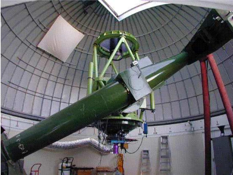
Figure 2.1: Photograph of the 1.3 m McGraw-Hill telescope of the MDM observatory located at Kitt Peak, Arizona. The long green-colored tube is the equatorial mount. Connected to this tube is the waffle-tree arrangement that supports the primary mirror, not seen in the photograph, and the secondary mirror, of diameter 0.5 m, on the top. Credits: Markus Böttcher
