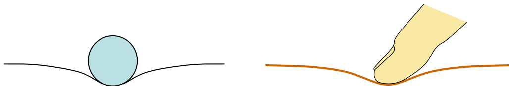
Figure 4.2 Deformation Due to a Finger is Similar to a Round Rigid Object
