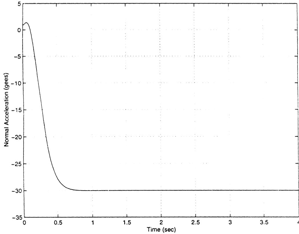
**Figure 4.3** Response of Nonlinear Closed-Loop System with State-Feedback Controller to -30g Normal Acceleration Command
