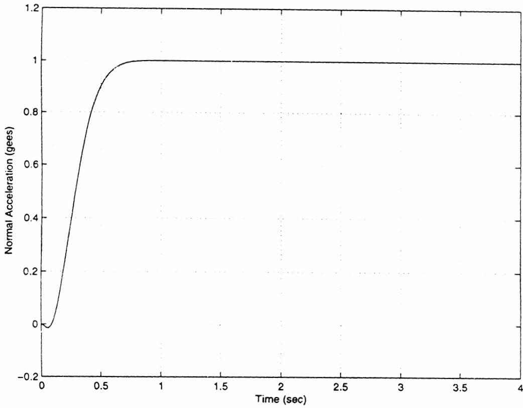
**Figure 4.2** Linear Closed-Loop Unit Step Response
