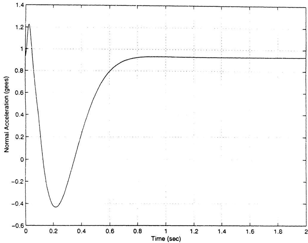
**Figure 4.7** Response of Nonlinear Closed-Loop System with Observer-Based Controller to Disturbance in the Reduced-Order Observer States
