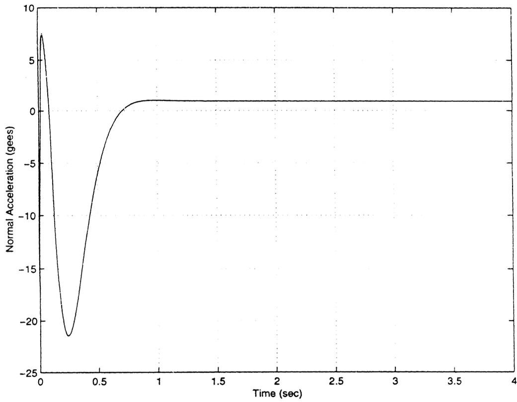
**Figure 4.5** Response of the Nonlinear Closed-loop System to the disturbance of the states
