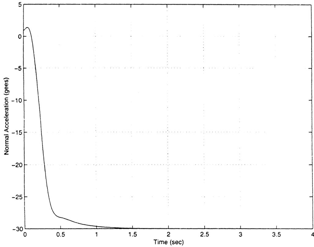
**Figure 4.4** Response of the System with Linear State-Feedback Controller to -30g Normal Acceleration Command
