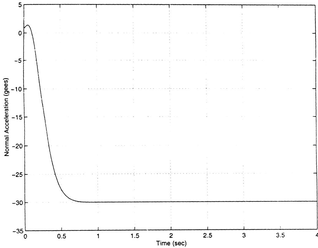
**Figure 4.6** Response of Nonlinear Closed-Loop System with Observer-Based Controller to -30g Normal Acceleration Command
