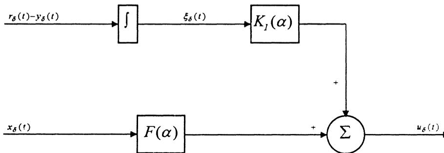
**Figure 2.2** Block Diagram of Parameterized Linear Controller (2.7)
