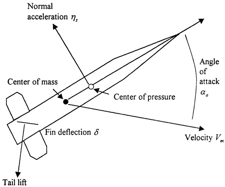
Figure 4.1 Pitch-axis missile
