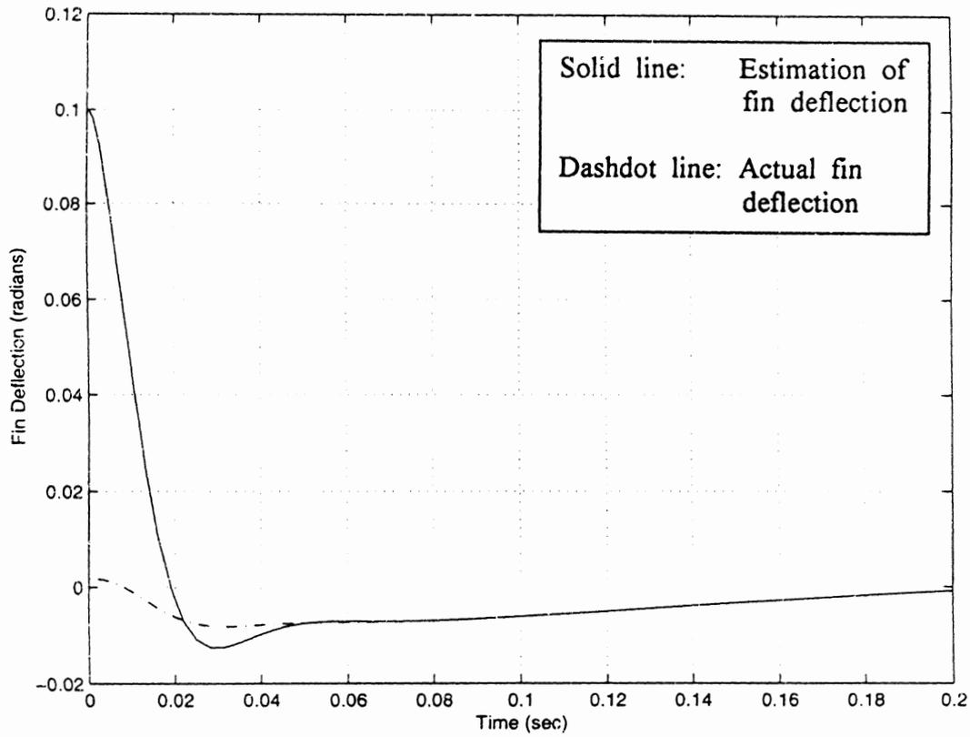
**Figure 4.8** Response of the Fin Deflection and its Estimation due to the Disturbance in the Reduced-Order Observer States
