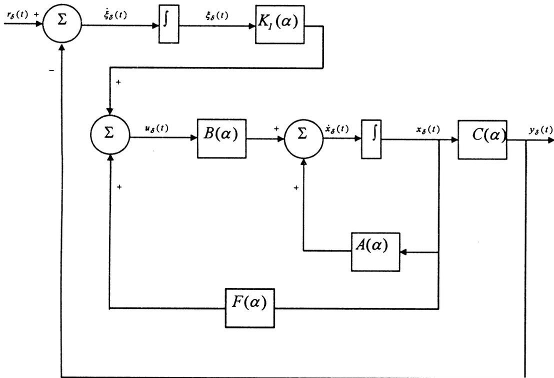
**Figure 2.1** Parameterized Linear Closed-Loop System
