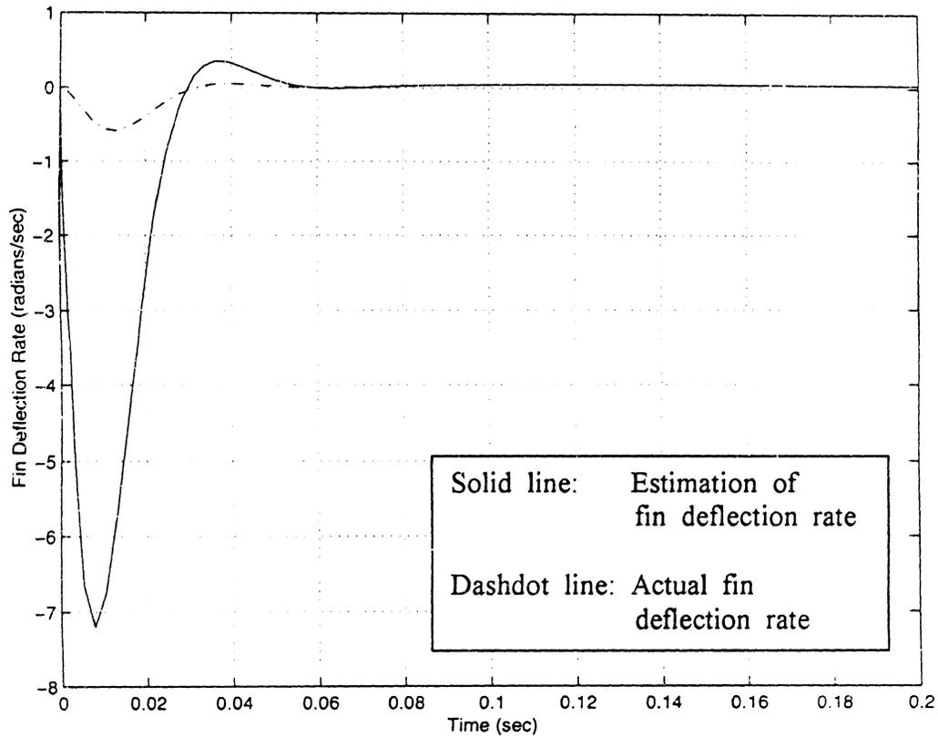
**Figure 4.9** Response of the Fin Deflection Rate and its Estimation due to the Disturbance in the Reduced-Order Observer States
