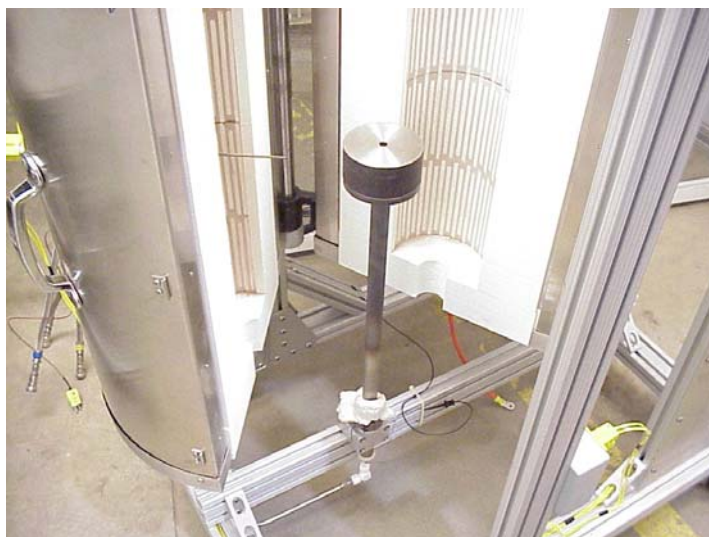
Figure 4.1 Placement of Anode Manifold into Single Cell Test Stand.
