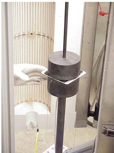
Figure 4.14 Final Placement of Cathode Manifold.
