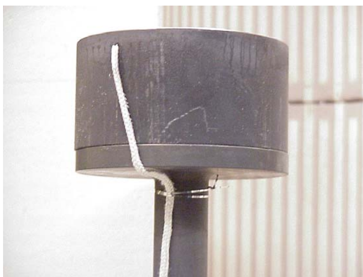
Figure 4.2 Positioning of Manifold Thermocouple.
