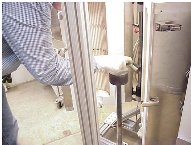
Figure 4.3 Layer of NiO Ink Being Applied to Anode Manifold.
