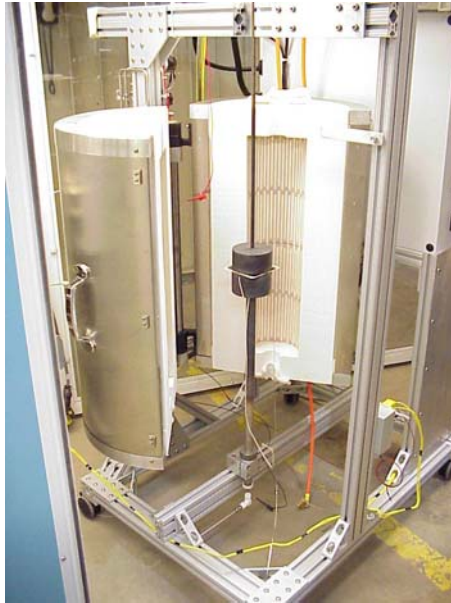
Figure 4.17 Single Cell Test Stand Ready to be Closed.
