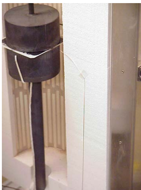
Figure 4.12 Cathode Voltage Tap Taped into Position.
