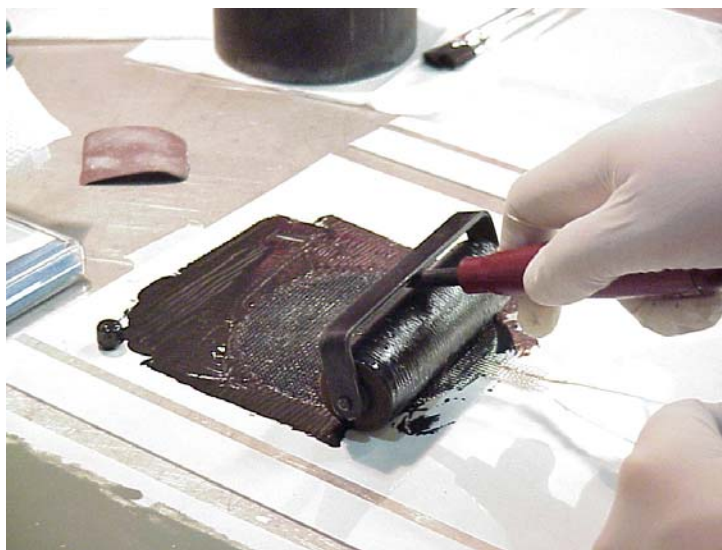
Figure 4.10 Rolling 0.8 PrO 8 Ink onto Silver Mesh.
