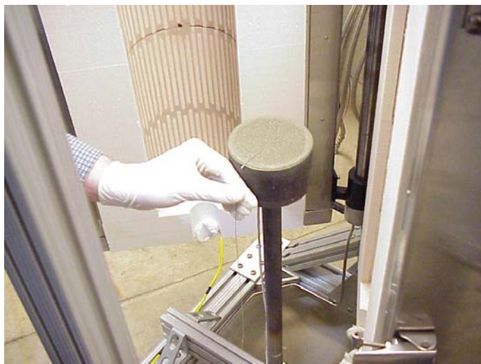
Figure 4.5 Placement of Incanel Ribbon onto Nickel Foam.
