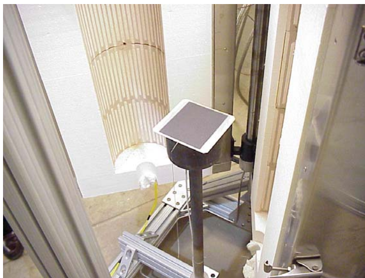
Figure 4.7 Placement of PSOFC onto Anode Manifold.
