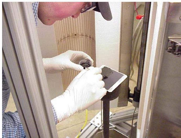
Figure 4.8 Application of 0.8 PrO 8 Ink to PSOFC Cathode.
