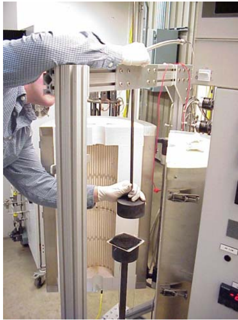
Figure 4.13 Positioning of Cathode Manifold.
