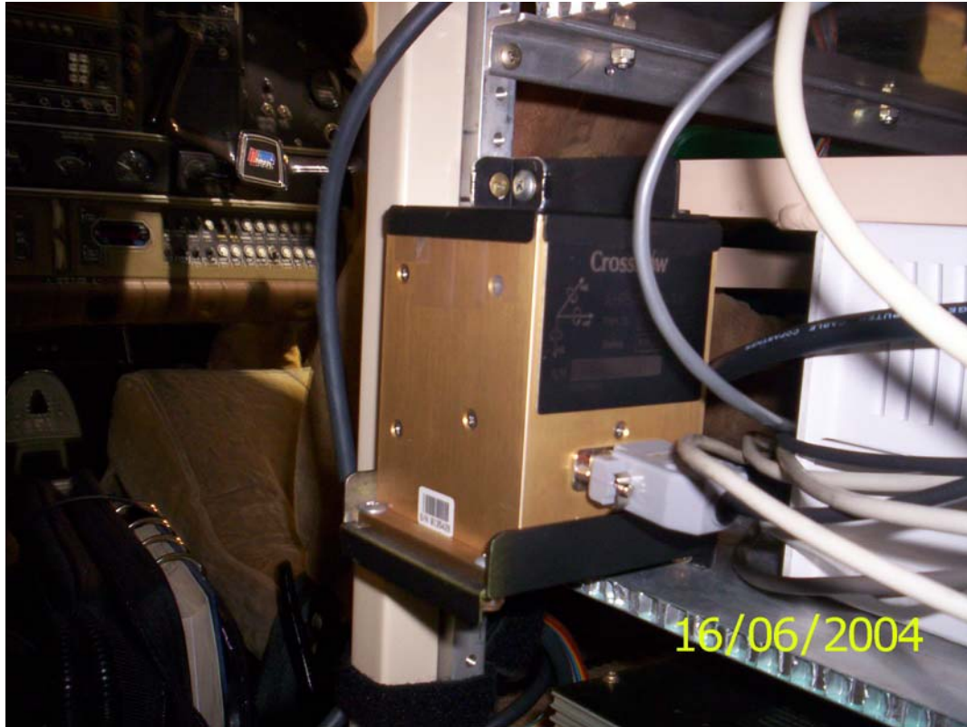
Figure 3.8: AHRS Mounted Near the CG of the Aircraft
