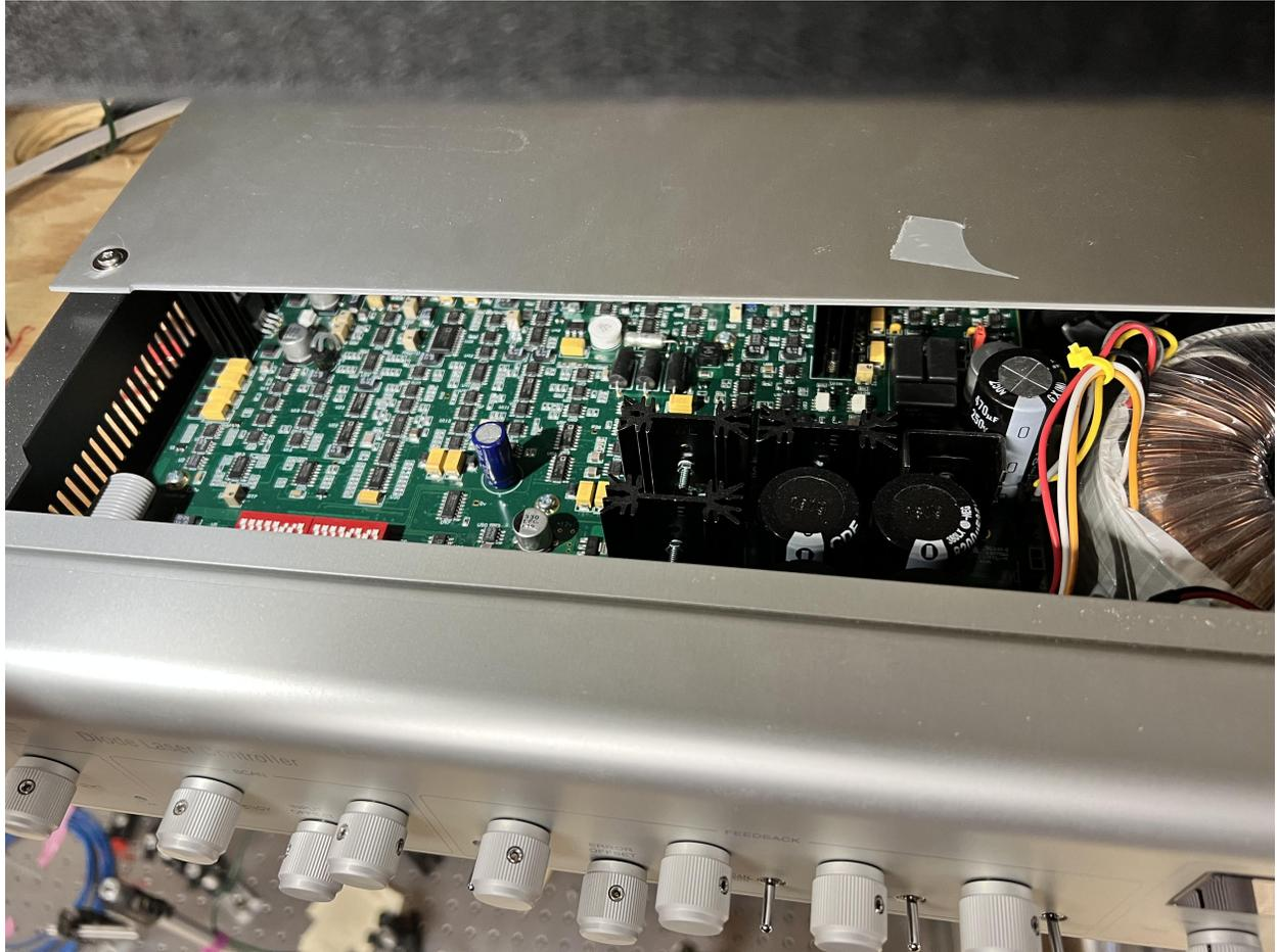
Figure A.1: Image of the inside of the DLC. The dipswitches are in the bottom left, a bright red panel. The BIAS dipswitch is the fourth from the right.
