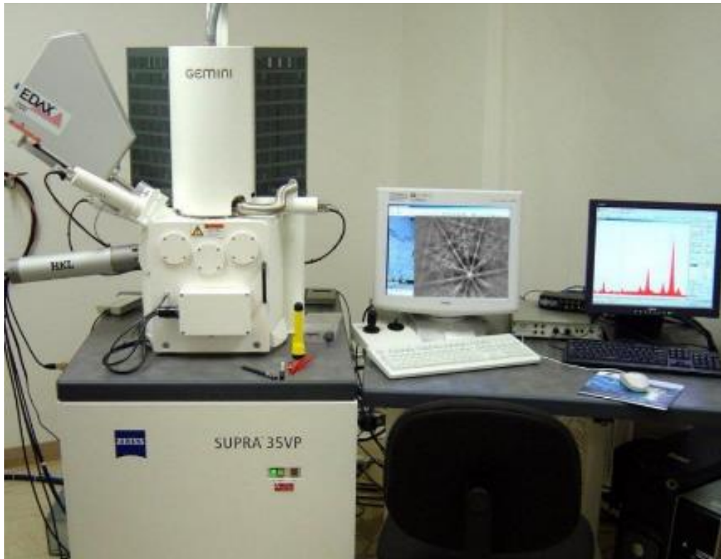
Fig. 3.5. The Scanning Electron Microscope (SEM) used for all the elemental analyses. It is housed in the Miami University Center for Advanced Microscopy and Imaging (CAMI), Zeiss Supra 35VP (variable pressure), X-ray fluorescence detector EDAX and HKL Electron Backscatter diffraction (EBSD) detector.
