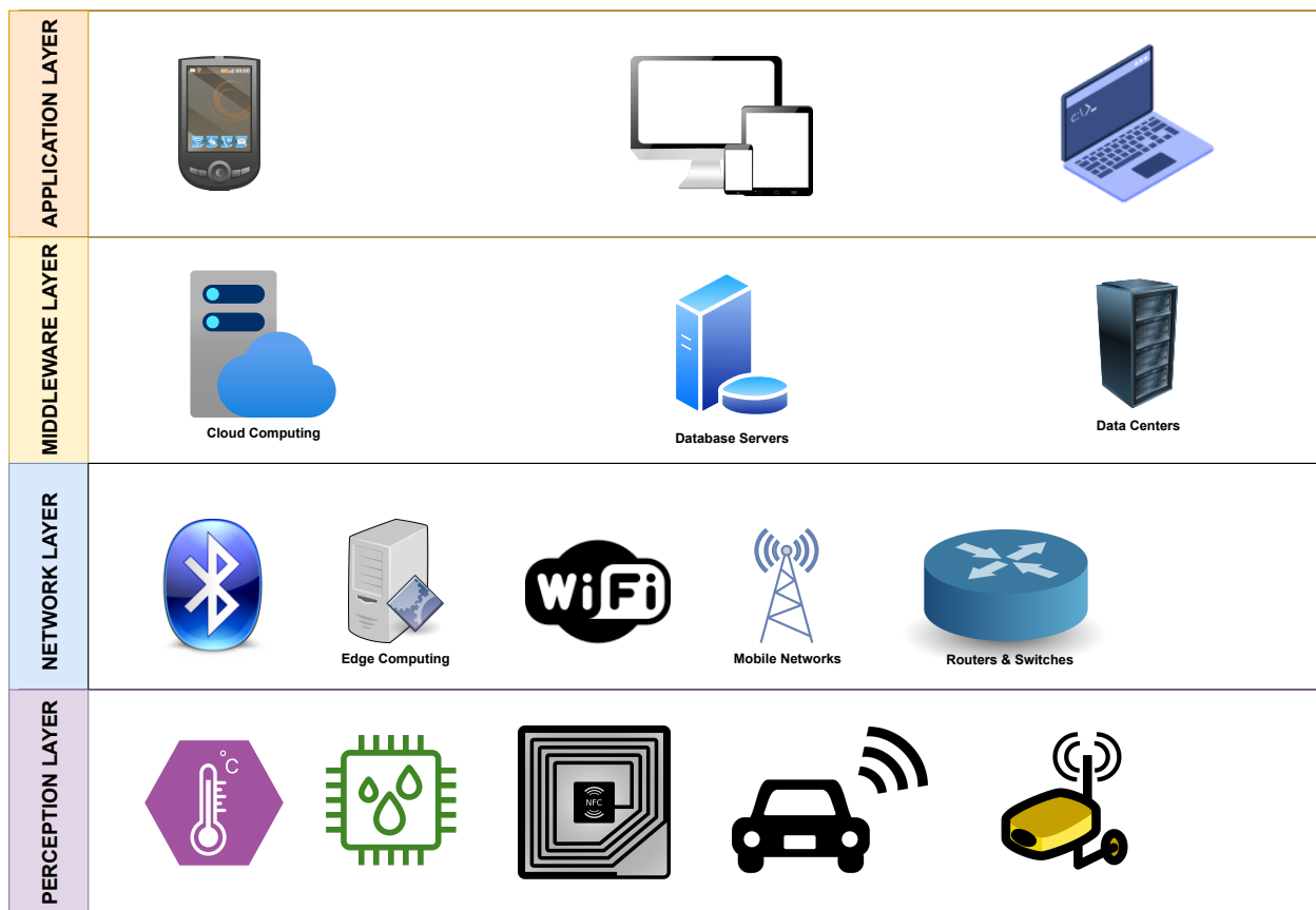
Figure 2.2: The 4 Layer IoT Architecture
