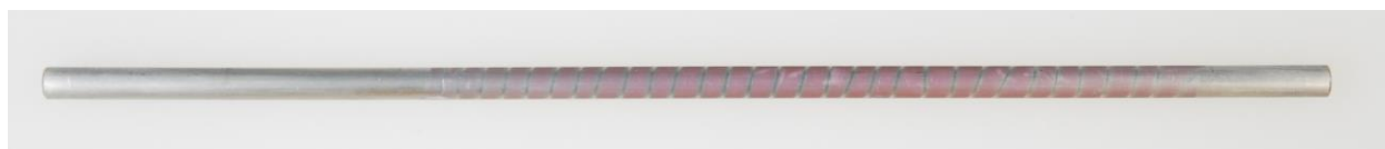
Figure 34. Picture of the patterned sample with hydrophobic silica nanospring regions (pink) adjacent to hydrophilic bare aluminum regions (gray).
