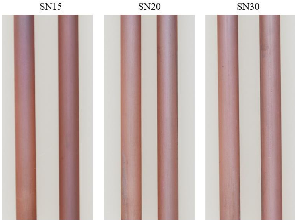
Figure 46. Pictures of untested (left) and tested (right) SN15, SN20, and SN30 samples for durability assessment.
