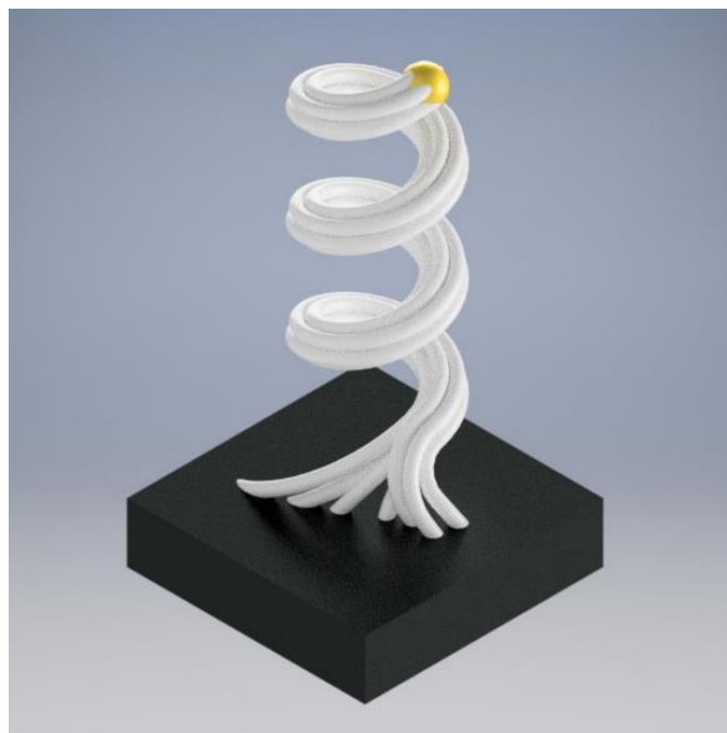
Figure 6. Rendering of a single nanowire structure showing multiple nanowires coming together and intertwining to form the nanospring.
