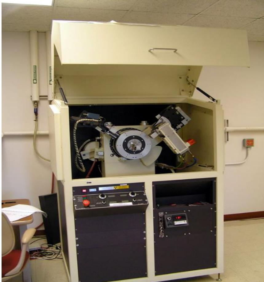
**Figure 3.2 Scintag x-ray diffractometer**
