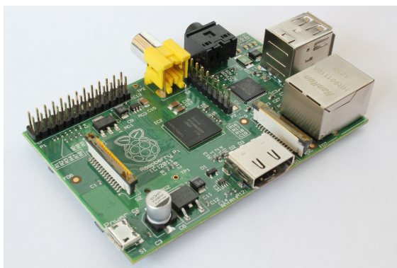
Figure 5.2: This is a Raspberry Pi and it provides the basis for our imager. It will be the component taking the image from the camera and displaying it on a touch screen
