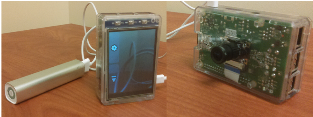
Figure 5.5: Image of the front on back of our IR viewer. We used a pre-made case and are in the process of modifying it.
