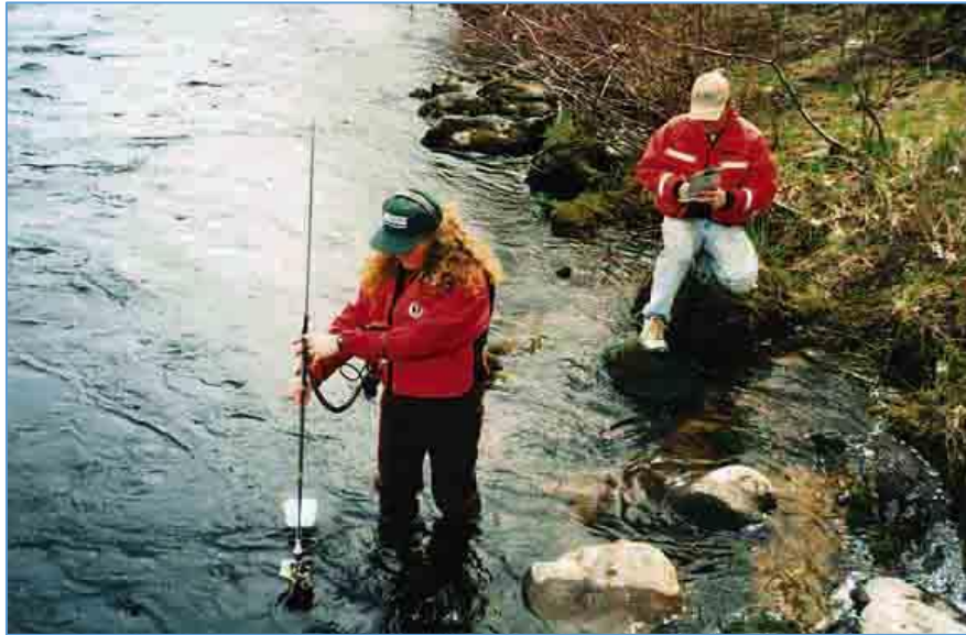
Figure 15: Use of a flowmeter in a stream. The sensor at the base of the pole is connected to a monitor that displays the speed of the stream current in feet per second. The flowmeter pole doubles as a depth measuring tool and is marked off in increments of either inches or centimeters (DeShon et al., 2015).
