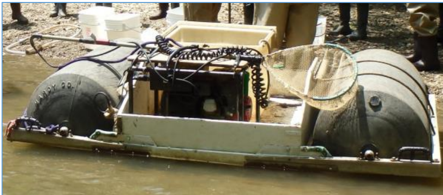
Figure 4: This vessel, a type of roller pram commonly referred to as a “Rollerbeast”, is used for wading electrofishing. A creation of the Ohio EPA, the Rollerbeast is composed of a metal frame with two plastic barrels for buoyancy. Electric current flows into the water directly from the anodes located on the rim of the net. Long-line electrofishing, done in small streams not deep enough for the wading method, uses a similar net-shocking set-up, only with the generator kept on land and connected with a long extension cord or “line” (DeShon et al., 2015).
