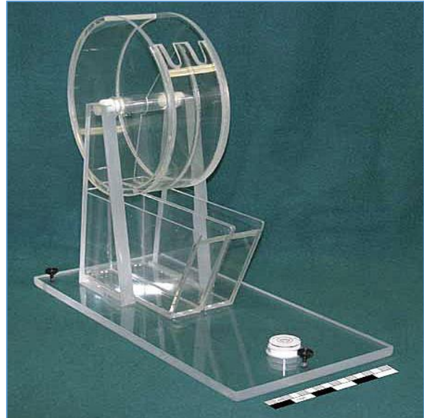
Figure 17: A Folsom sample splitter is used to create subsamples of macroinvertebrates. All components are clear to ensure adequate distribution of the sample before splitting (Anderson, 2004).
