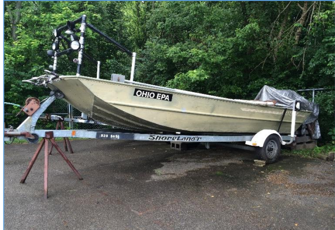
Figure 3: The electrofishing boat rig used by the Ohio EPA. Operators use a foot pedal on the bow of the boat to initiate the output of electric current. Current flows into the water from anodes suspended from a boom that extends out in front of the bow (Photo by Rebecca Long).
