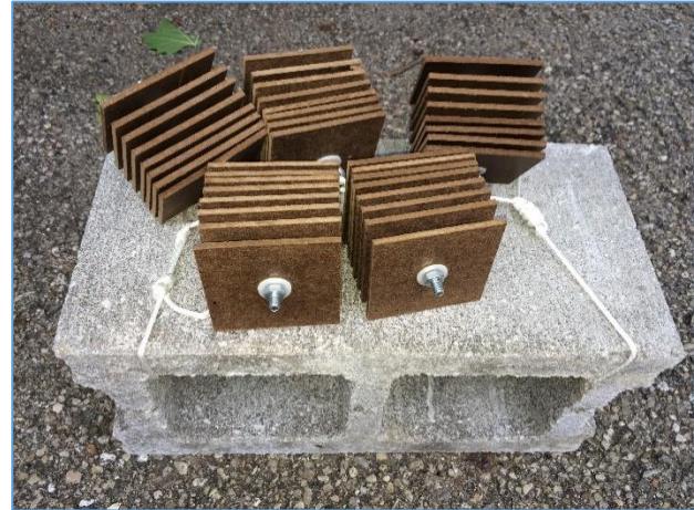
Figure 5: Hester-Dendy multiplate artificial substrate samplers. Each sampler block is composed of eight pieces of Masonite hardboard separated in various widths by nylon spacers (Photo by Rebecca Long).
