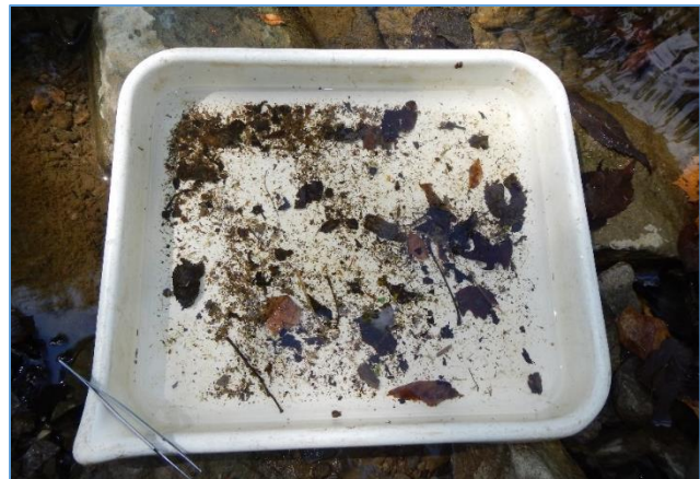
Figure 13: The white pan used for picking organisms out of stream debris. The contrast provided the white bottom makes organisms easier to see (DeShon et al., 2015).
