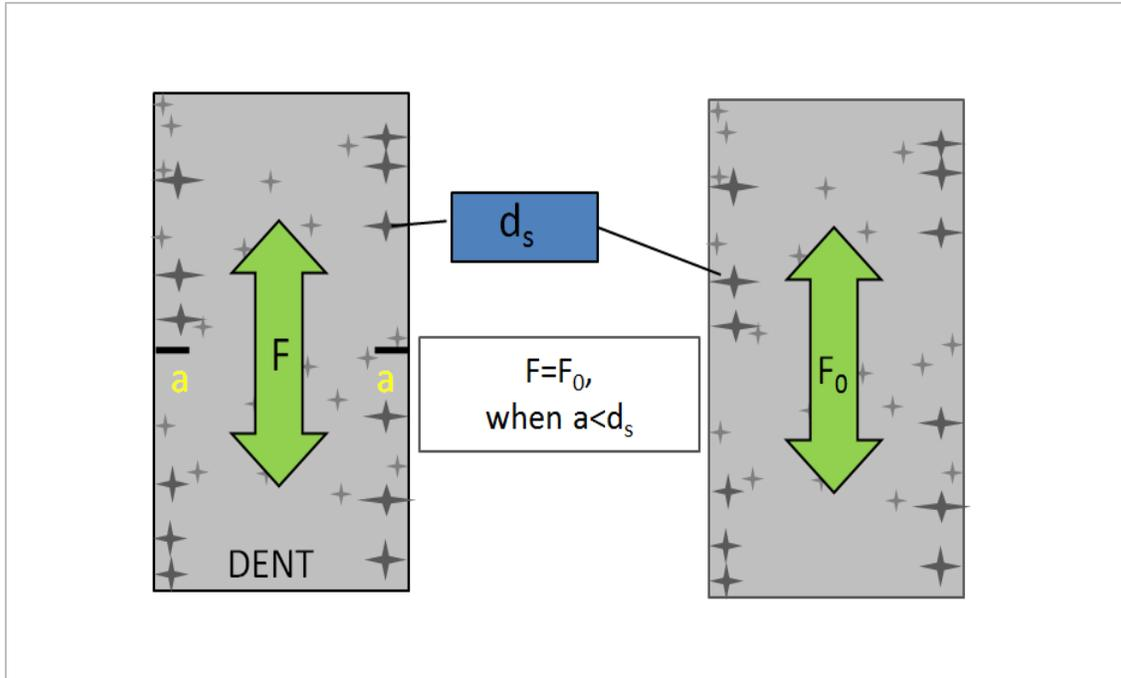
**Figure 7 DENT specimen with small notches shows notch insensitivity character**
