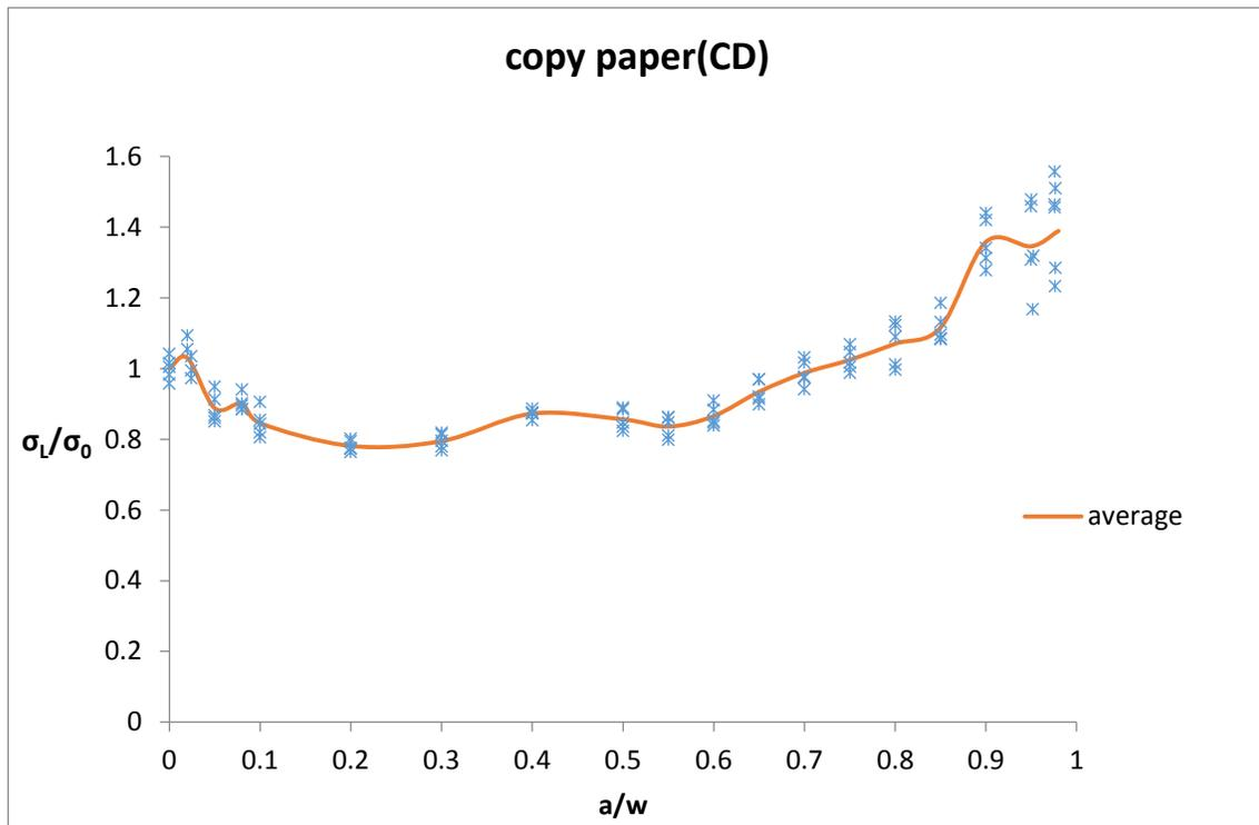
**Figure 13 Average ligament stress normalized by tensile strength for CD copy paper. Red line represents the average value of the experimental data**
