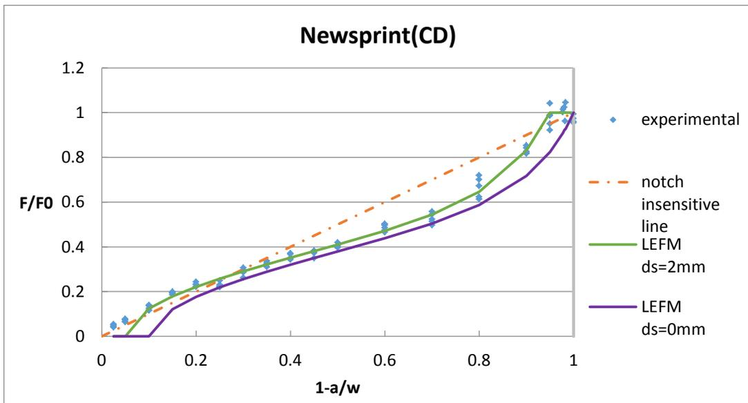
**Figure 24 DENT load ratios versus relative ligament length for newsprint CD direction.**
