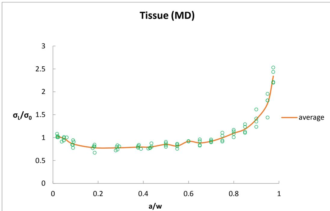
**Figure 19 Average ligament stress normalized by tensile stress for MD tissue paper. Red line represents the average value of the experimental data and trend line is also plotted.**
