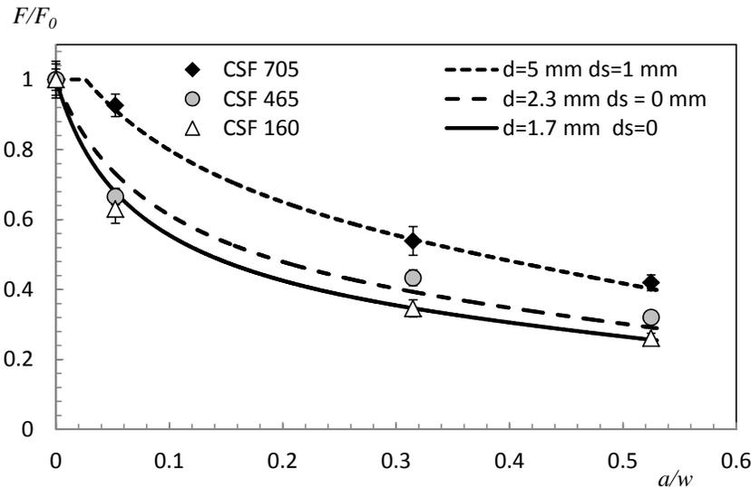
Figure 21. Effect of beating on DENT fracture sensitivity for handsheets, 50 g/m<sup>2</sup>.
