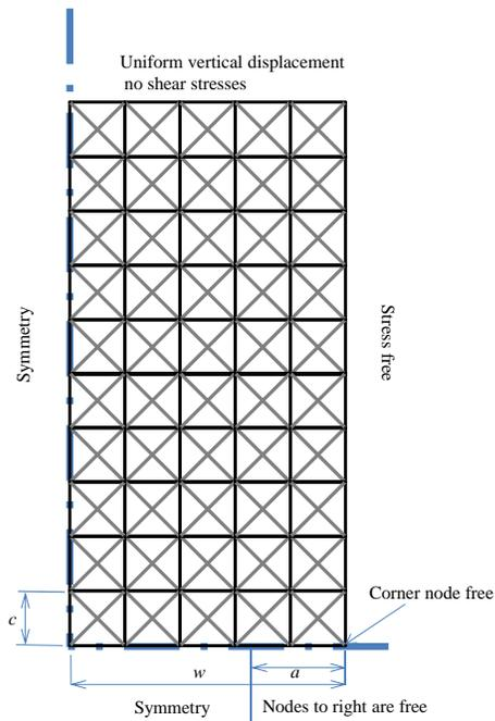
Figure 3. Flawed Lattice model (1/4 of DENT specimen)
