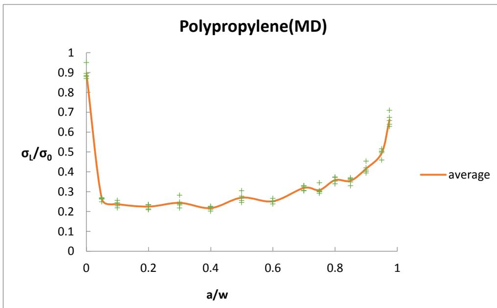
**Figure 22 Average ligament stress normalized by tensile strength for MD polypropylene film. Red line represents the average value of the experimental data**
