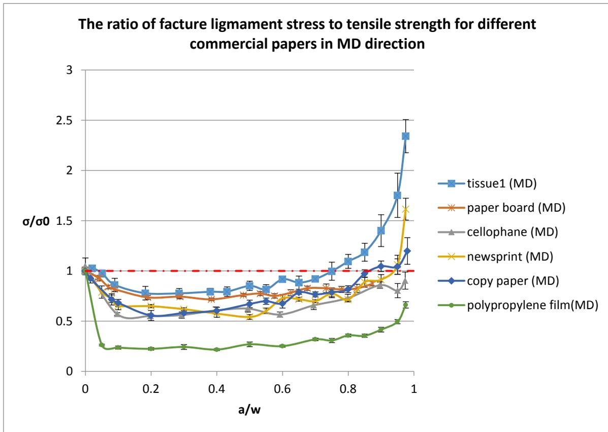
**Figure 23 The ratios of ligament stress to tensile strength for different commercial papers in MD direction**
