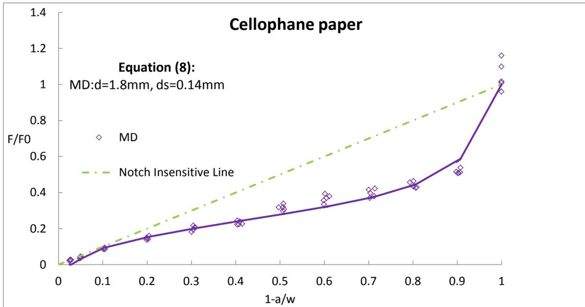
**Figure 9 DENT load ratio versus relative ligament length for cellophane film MD direction. The solid lines are the Equation (8) and the dash line is notch-insensitive line.**
