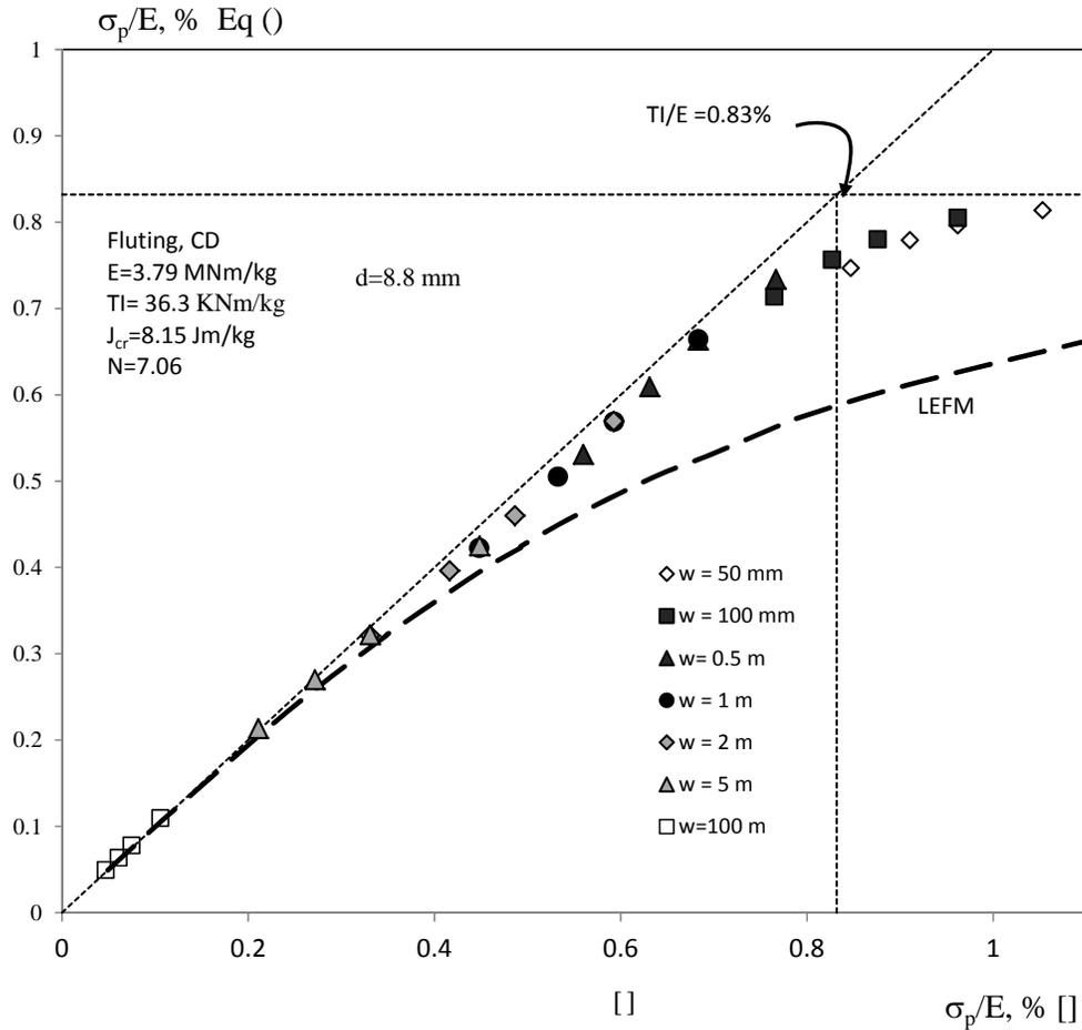
Figure 13. Comparison of Equation (6) with that from Reference [17] for CD Fluting.
