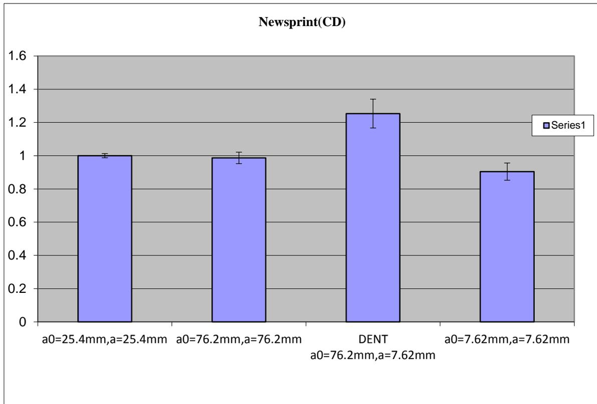
**Figure 27 Comparison of average ligament stress versus tensile strength of deeply notched DENT specimen for CD newsprint paper**
