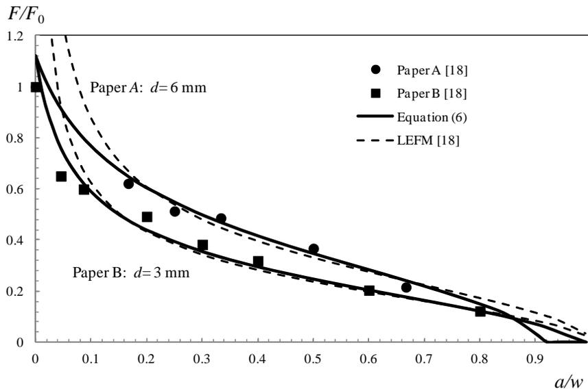
Figure 10. Comparison of Equation (6) to LEFM using data from [18].
