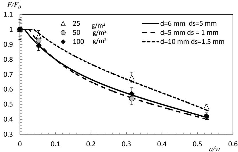
Figure 23. Influence of grammage on fracture sensitivity of handsheets from unbeaten pulp.
