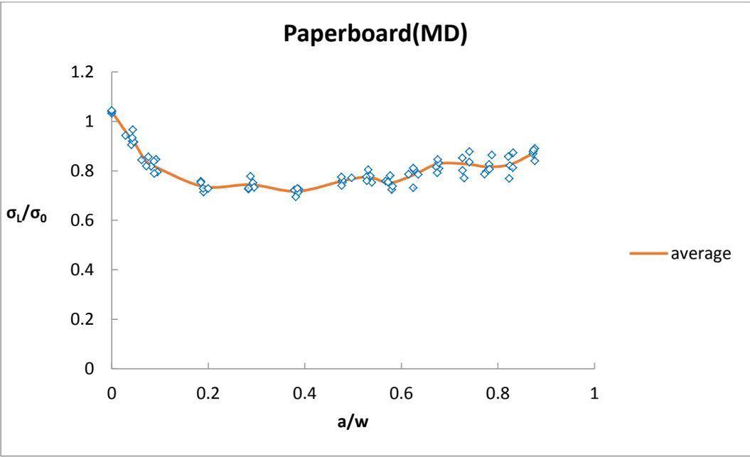
**Figure 20 Average ligament stress normalized by tensile strength for MD paperboard. Red line represents the average value of the experimental data**
