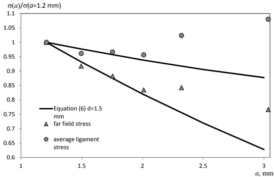
Figure 9. Relative far field stress level and average ligament stress for data from [10].
