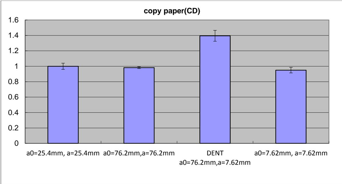
**Figure 25 Comparison of average ligament stress versus tensile strength of deeply notched DENT specimen for CD copy paper**
