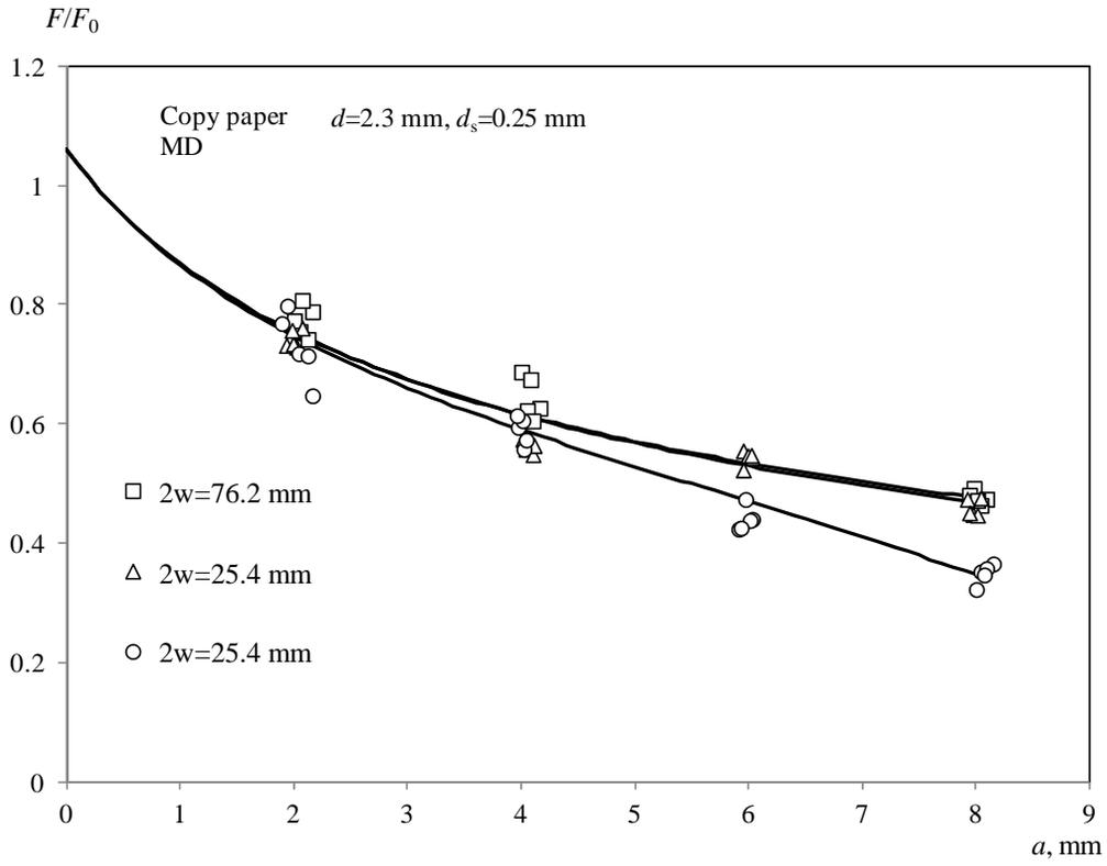
Figure 24. Fracture versus crack length for three widths. MD copy paper.
