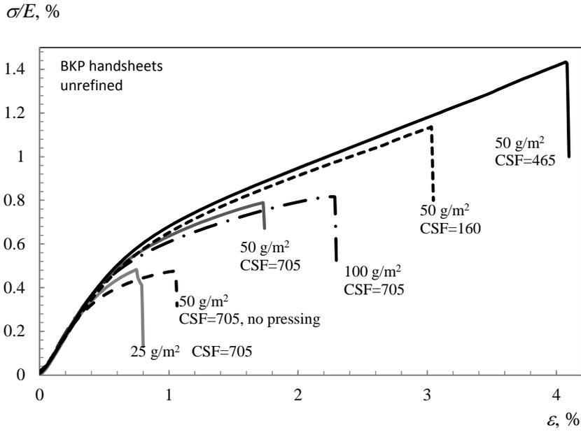
Figure 16. Stress-strain curves for handsheets.
