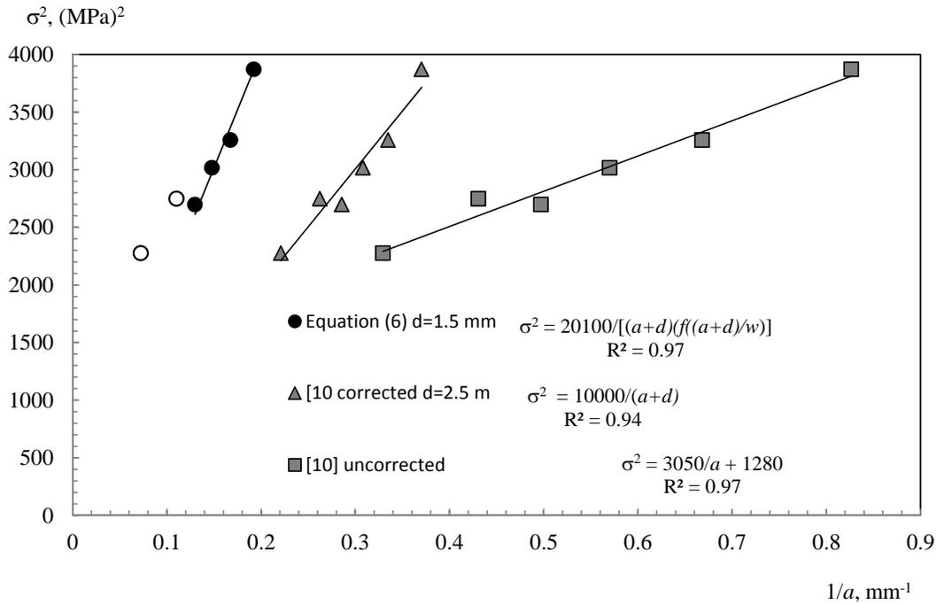
Figure 8. Fracture results from Fig 4 of Ref. [10] and Equation (6) with  $d=2.5$  mm.
