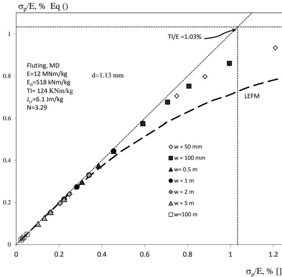
Figure 12. Comparison of Equation (6) with that from Reference [17] for MD Fluting.
