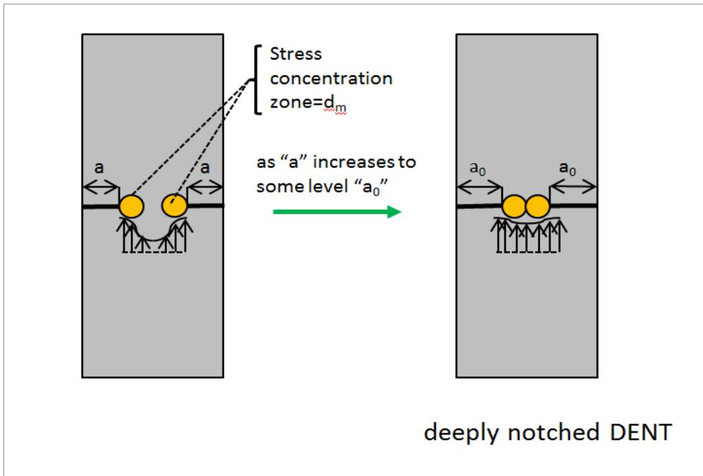
**Figure 6 deeply notched DENT specimen shows notch insensitivity character**
