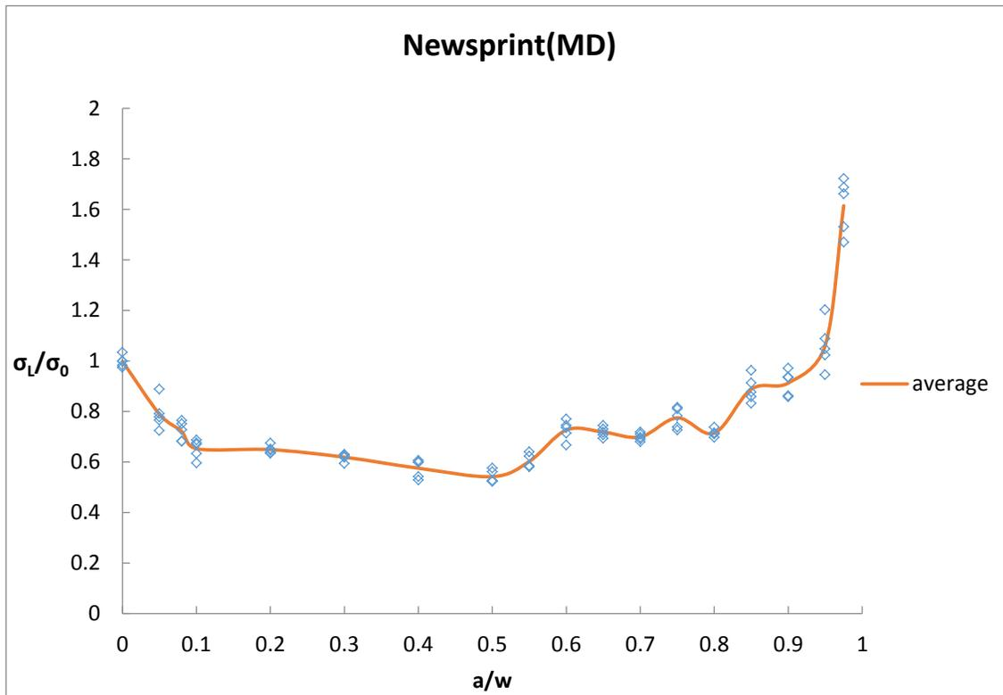
**Figure 17 Average ligament stress normalized by tensile strength for MD newsprint paper. Red line represents the average value of the experimental data**
