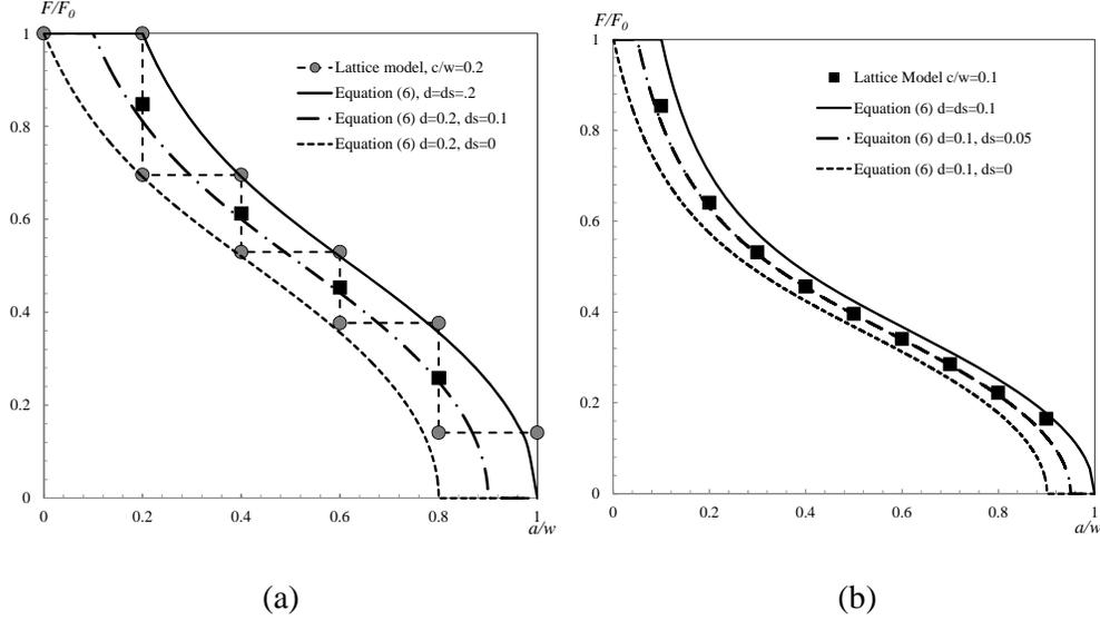
Figure 4. Load ratio versus crack length for flawed lattice model. Black squares represent the average load ratio that occurs before and after the release of a node at a crack length of  $a$ . (a) is for a lattice with  $w=5c$  and  $L=50c$ , and (b) is for  $w=10c$  and  $L=100c$ .
