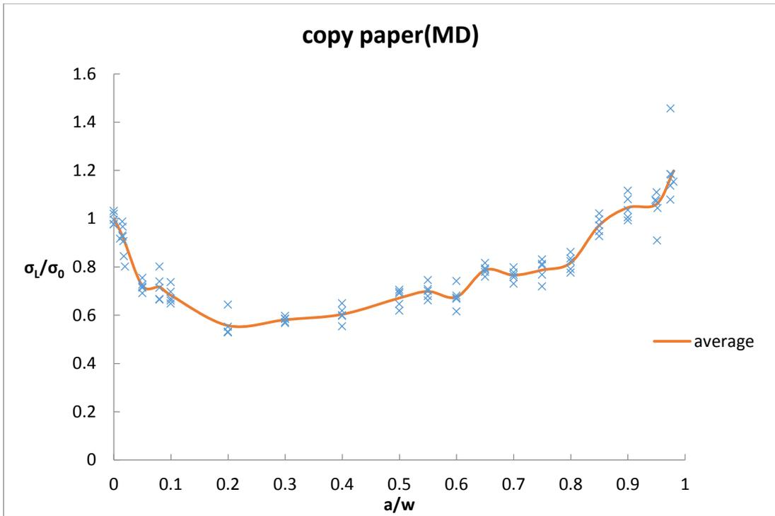
**Figure 14 Average ligament stress normalized by tensile strength for MD copy paper. Red line represents the average value of the experimental data**
