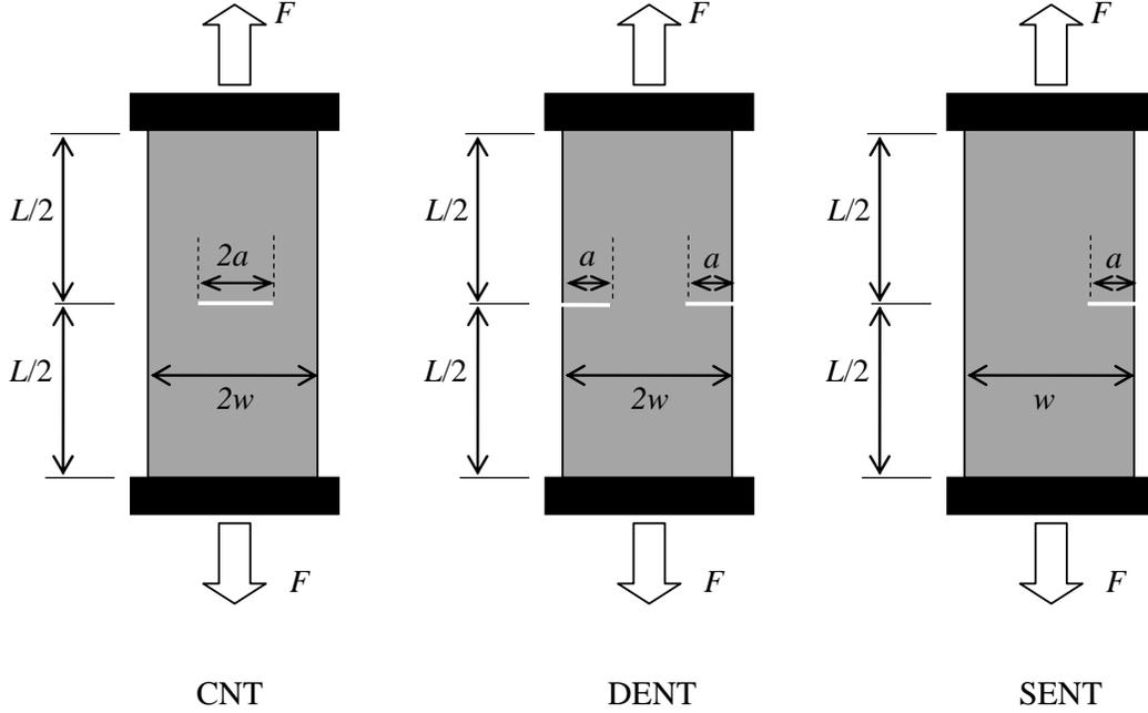
**Figure 1.** Typical geometries for in-plane fracture tests with paper.
