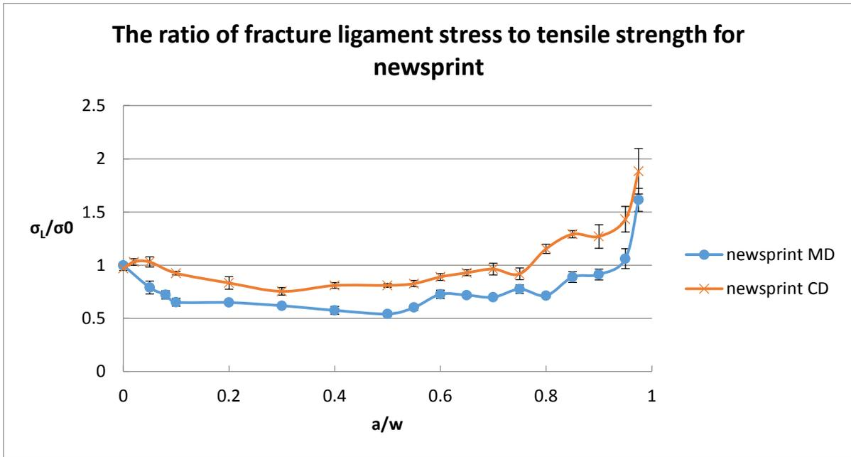
**Figure 18 The ratio of fracture ligament stress to tensile strength for newsprint in both machine direction and cross machine direction**
