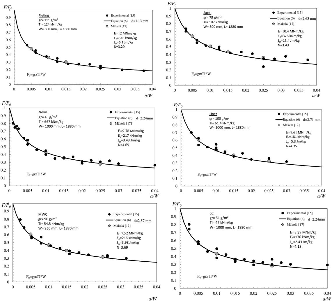
Figure 11. Comparison of LEFM results to experimental results from large webs [15], and the nonlinear fracture mechanics approach in [17].
