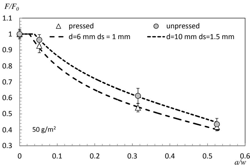
Figure 22. Effect of pressing on fracture sensitivity of handsheets made from unbeaten pulp.
