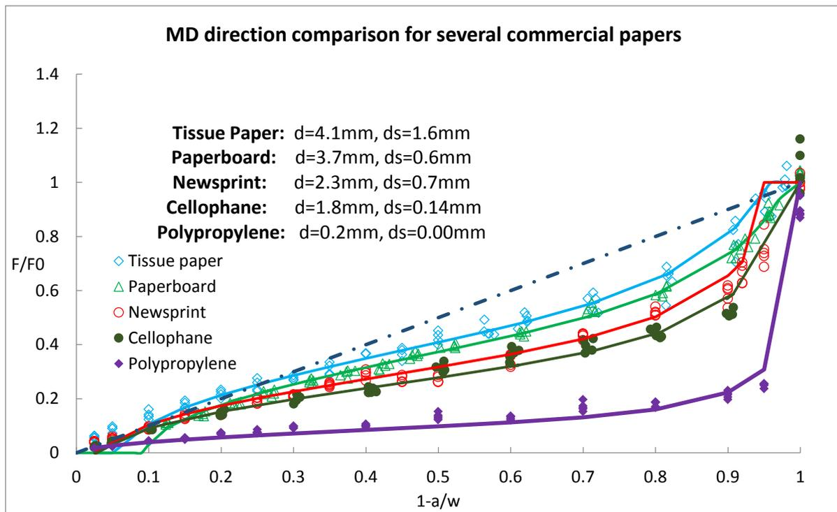
**Figure 12** The comparison for several commercial papers in MD direction. The solid lines are the Equation (8) and the dash line is notch-insensitive line.
