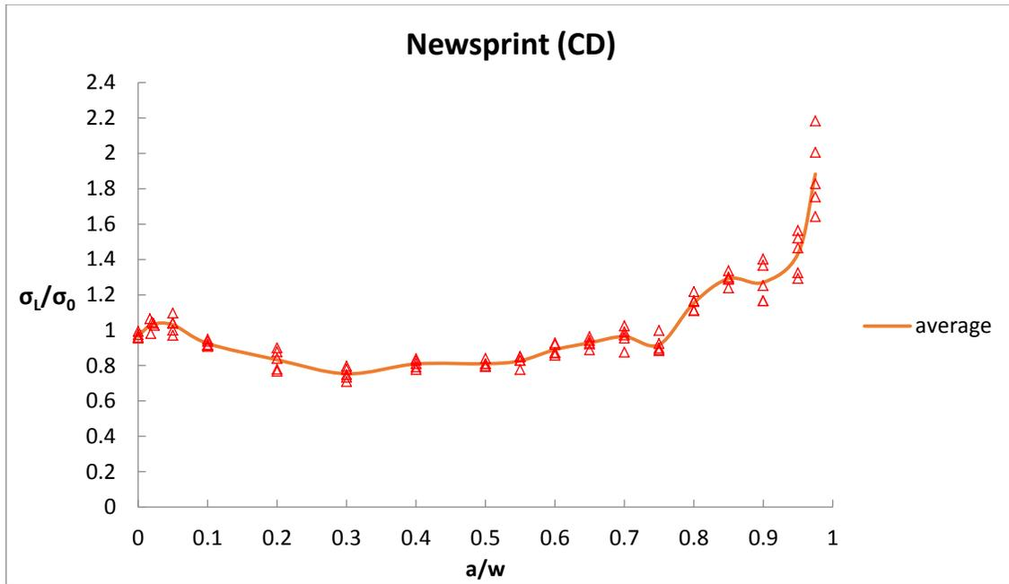
**Figure 16 Average ligament stress normalized by tensile strength for CD newsprint paper. Red line represents the average value of the experimental data**
