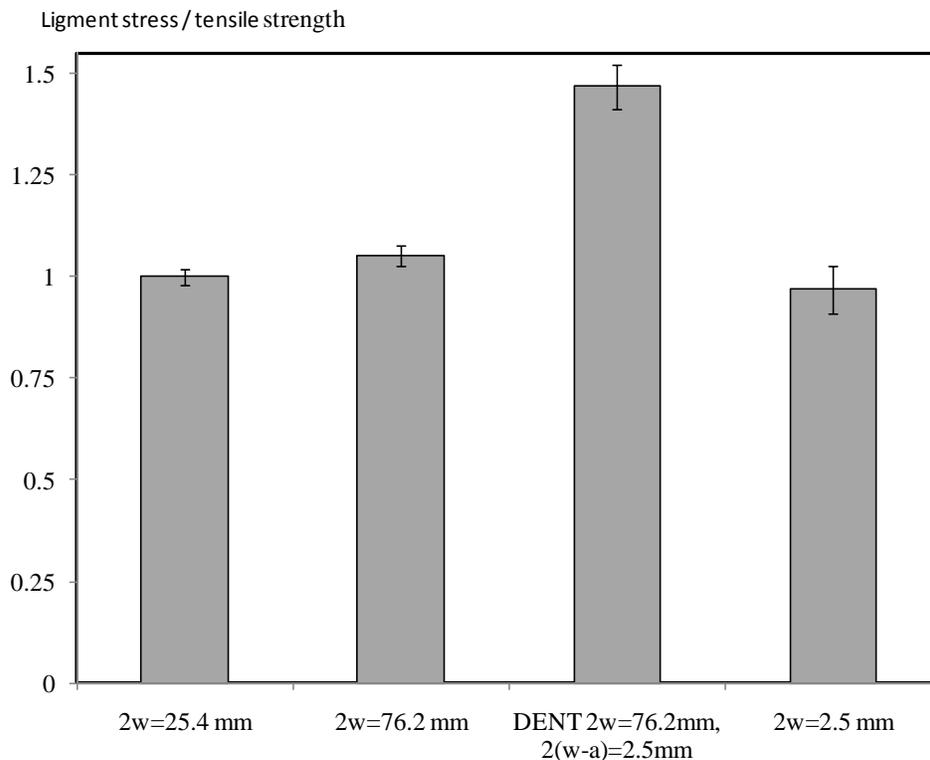
Figure 26. Comparison of tensile strength versus deep-notched DENT strength for MD copy paper.
