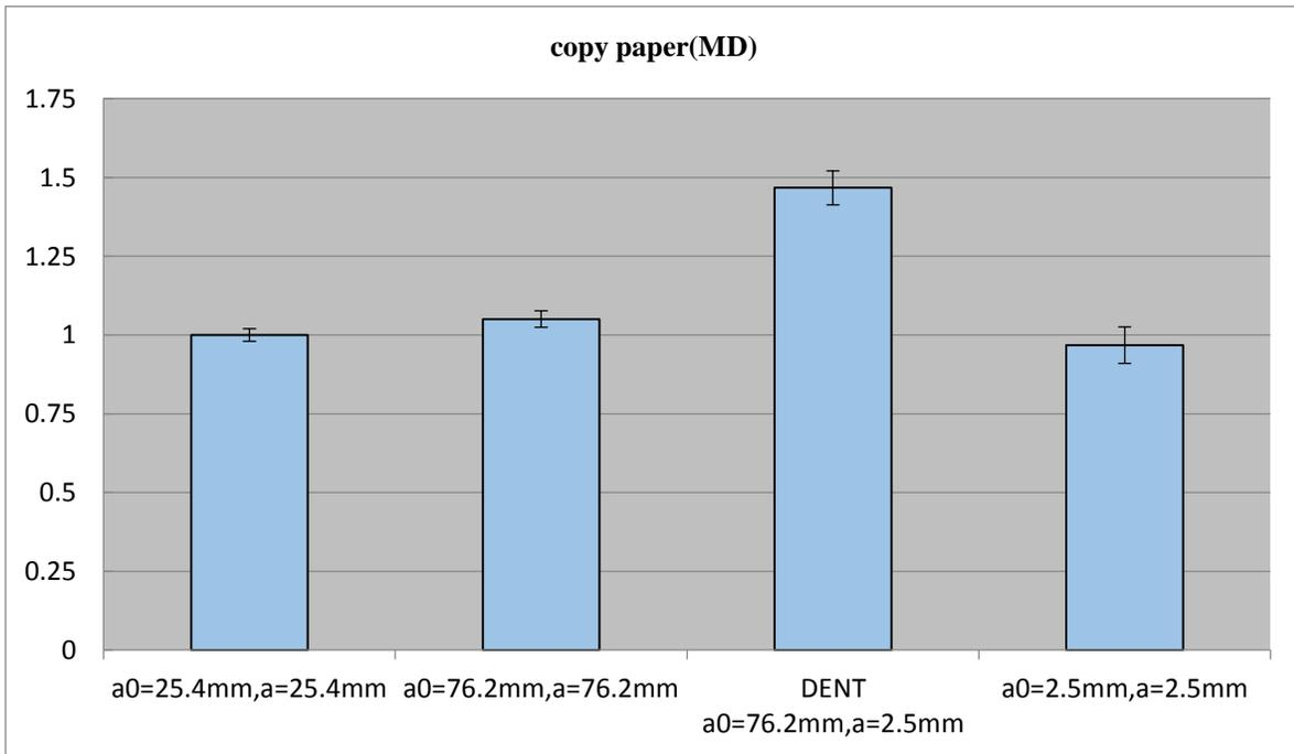
**Figure 26 Comparison of average ligament stress versus tensile strength of deeply notched DENT specimen for MD copy paper**
