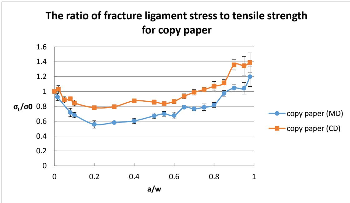
**Figure 15 The ratios of fracture ligament stress to tensile strength for copy paper in both machine direction and cross machine direction**
