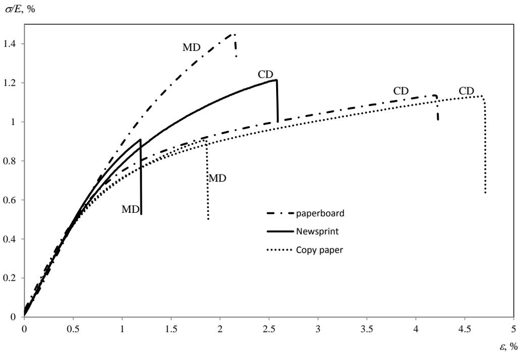
Figure 14. MD and CD Stress-strain curves for commercial papers. Stress is normalized to Elastic modulus.
