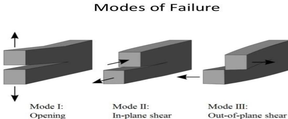
**Figure 1 The Three modes of Fracture**
