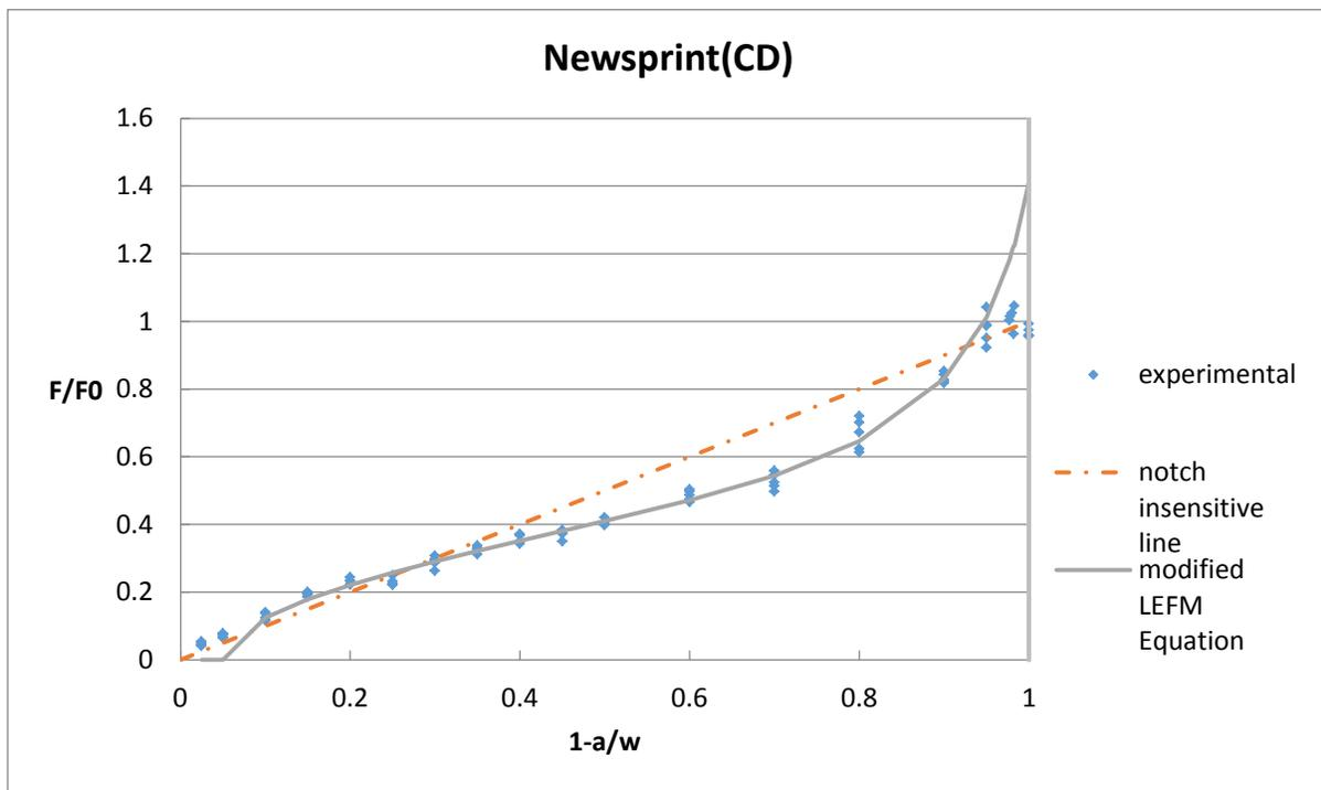
**Figure 30 Fracture load ratios versus ligament to width ratio for DENT specimen of CD newsprint,  $d_s=0\text{mm}$ .**
