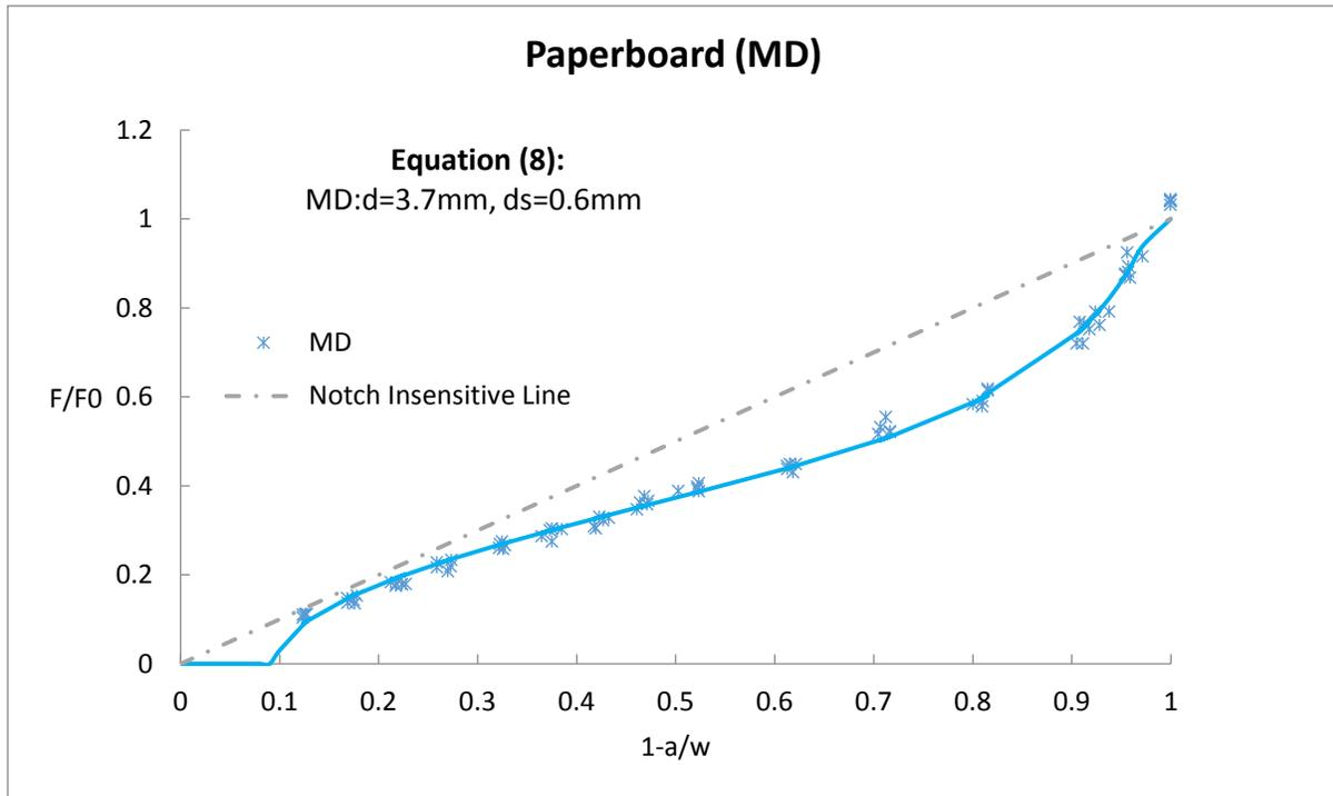
**Figure 10 DENT load ratio versus relative ligament length for paperboard in MD direction. The solid lines are the Equation (8) and the dash line is notch-insensitive line.**
