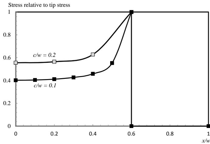
Figure 6. Stress distribution along ligament for two characteristic lattice sizes.
