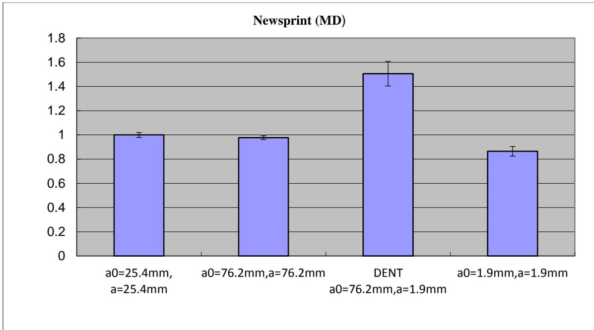
**Figure 28 Comparison of average ligament stress versus tensile strength of deeply notched DENT specimen for MD newsprint**
