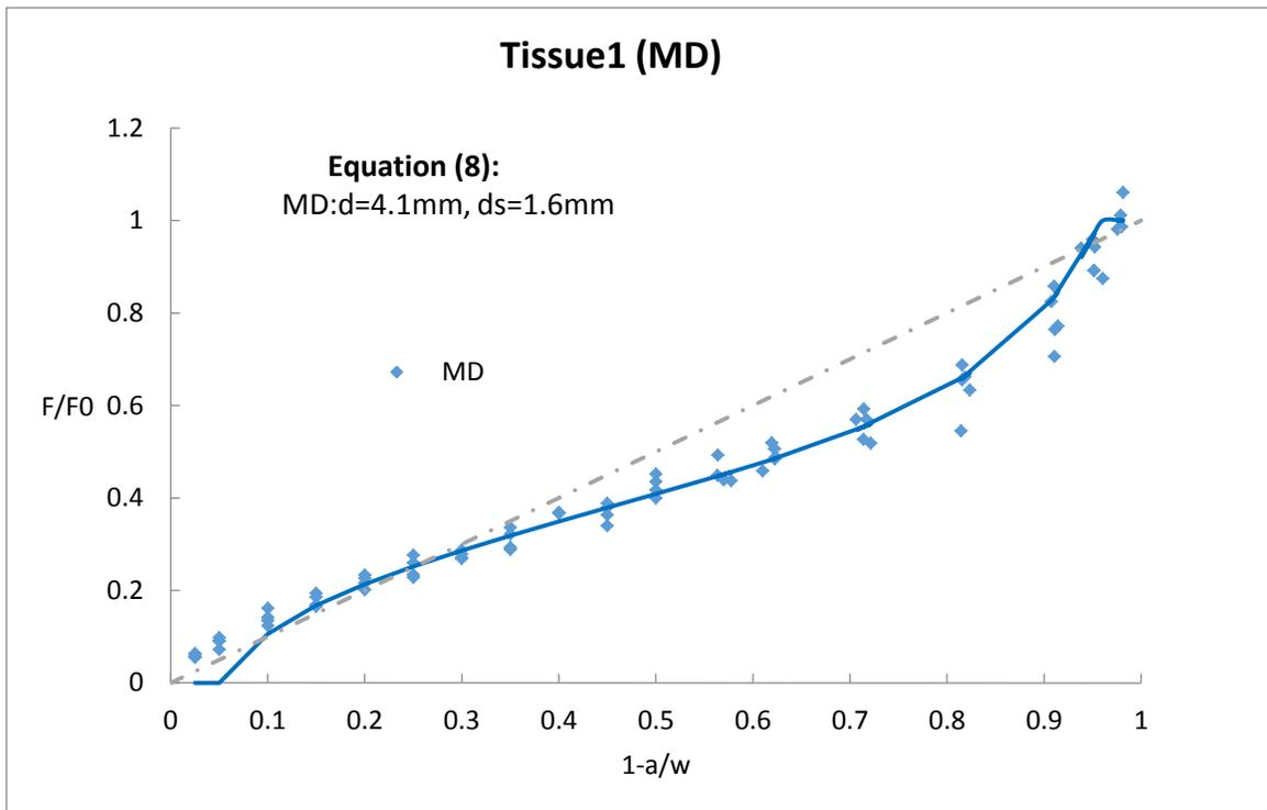
**Figure 8 DENT load ratio versus relative ligament length for Tissue MD direction. The solid lines are the Equation (8) and the dash line is notch-insensitive line.**
