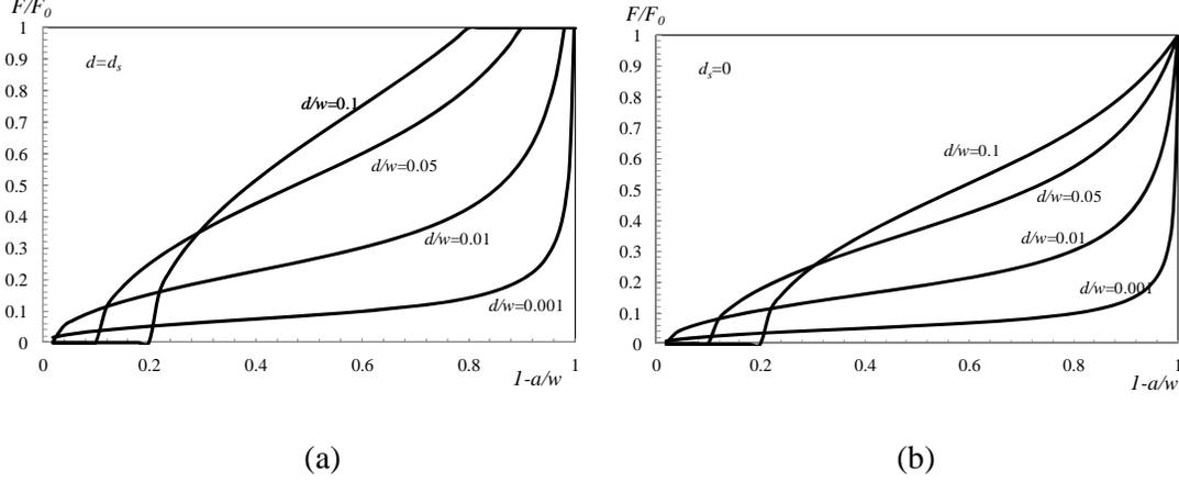
Figure 2. Fracture load ratio as a function of ligament length for various characteristic fracture lengths for DENT. (a) All structural  $d=d_s$ , (b) all material  $d_s=0$ .
