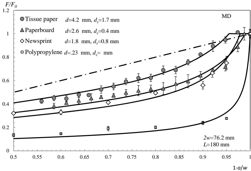
Figure 19. DENT results of load ratio versus relative ligament length for various papers in MD direction. Solid lines represent Equation (6). Dash-dot line represents notch-insensitive response  $F/F_0=1-a/w$ .
