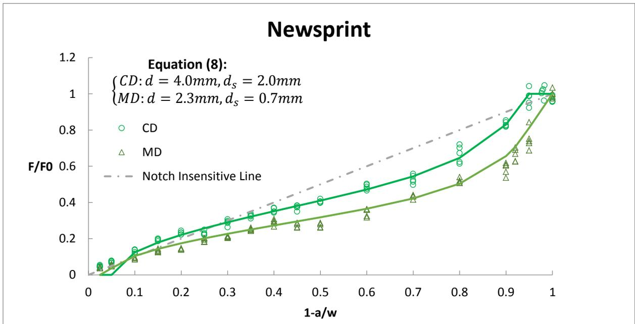
**Figure 5 DENT load ratio versus relative ligament length for newsprint. The solid lines are the Equation (8) and the dash line is notch-insensitive line.**
