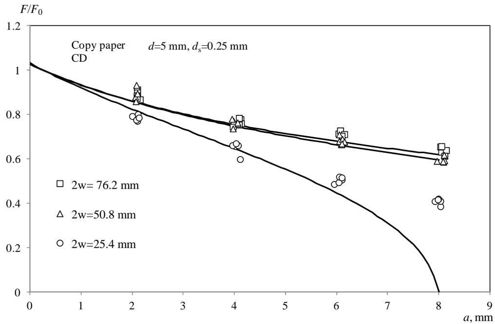
Figure 25. Fracture load versus crack length for three widths. Copy Paper CD
