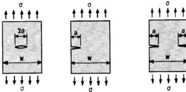
**Figure 2 Three Notch Geometries of Mode I Fracture[1]**
