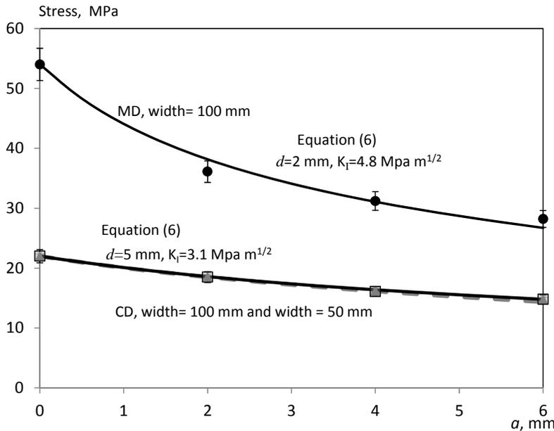
Figure 7. DENT fracture tests of a copy paper [6] compared to Equation (6).
