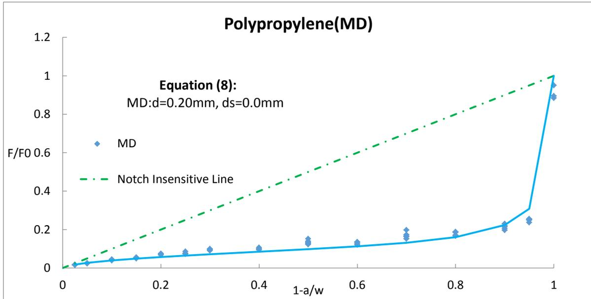
**Figure 11 DENT load ratio versus relative ligament length for polypropylene film in MD direction. The solid lines are the Equation (8) and the dash line is notch-insensitive line.**
