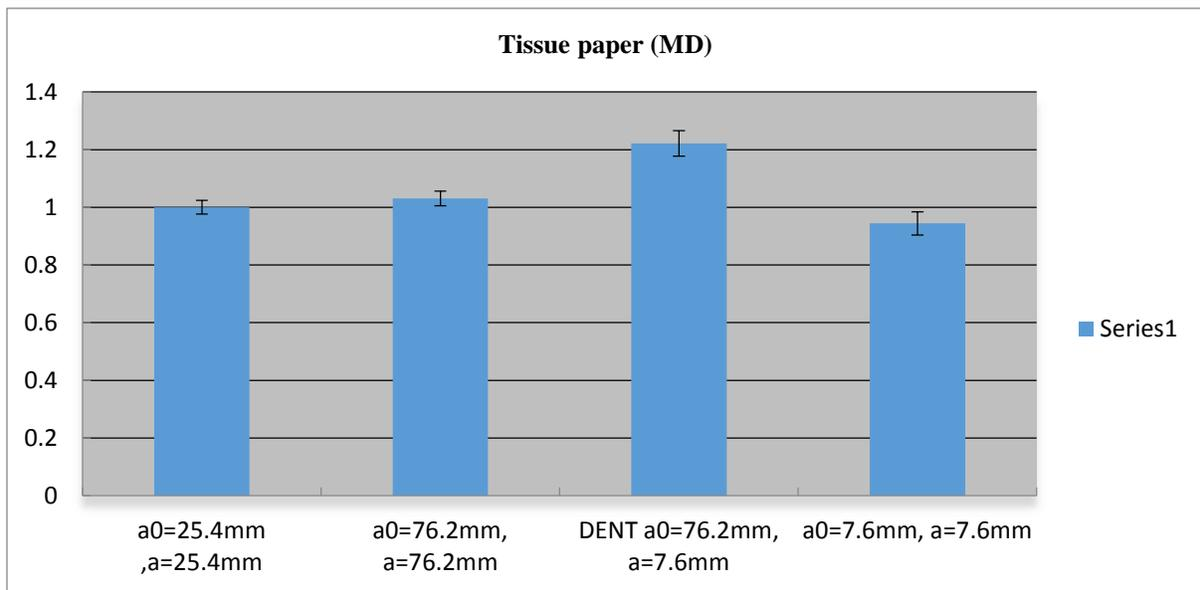
**Figure 29 Comparison of average ligament stress versus tensile strength of deeply notched DENT specimen for MD tissue paper**
