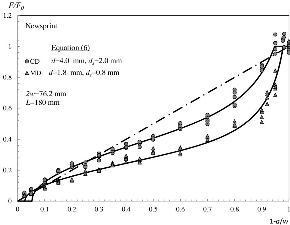
Figure 18. DENT results of load ratio versus relative ligament length for Newsprint. Solid lines represent Equation (6). Dash-dot line represents notch-insensitive response  $F/F_0=1-a/w$ .
