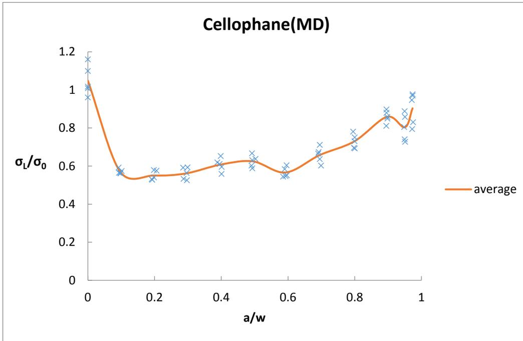
**Figure 21 Average ligament stress normalized by tensile strength for MD regenerated cellophane. Red line represents the average value of the experimental data**
