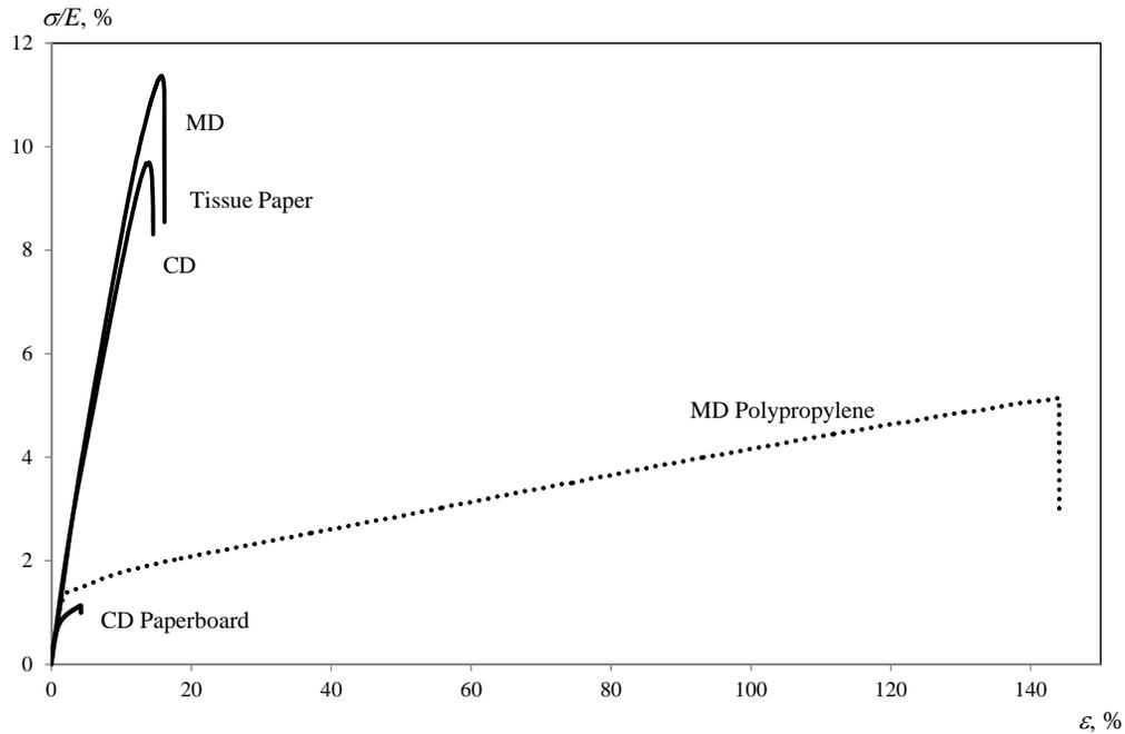
Figure 15. Stress-strain curves for tissue paper and polypropylene film. Stress is normalized to Elastic modulus.
