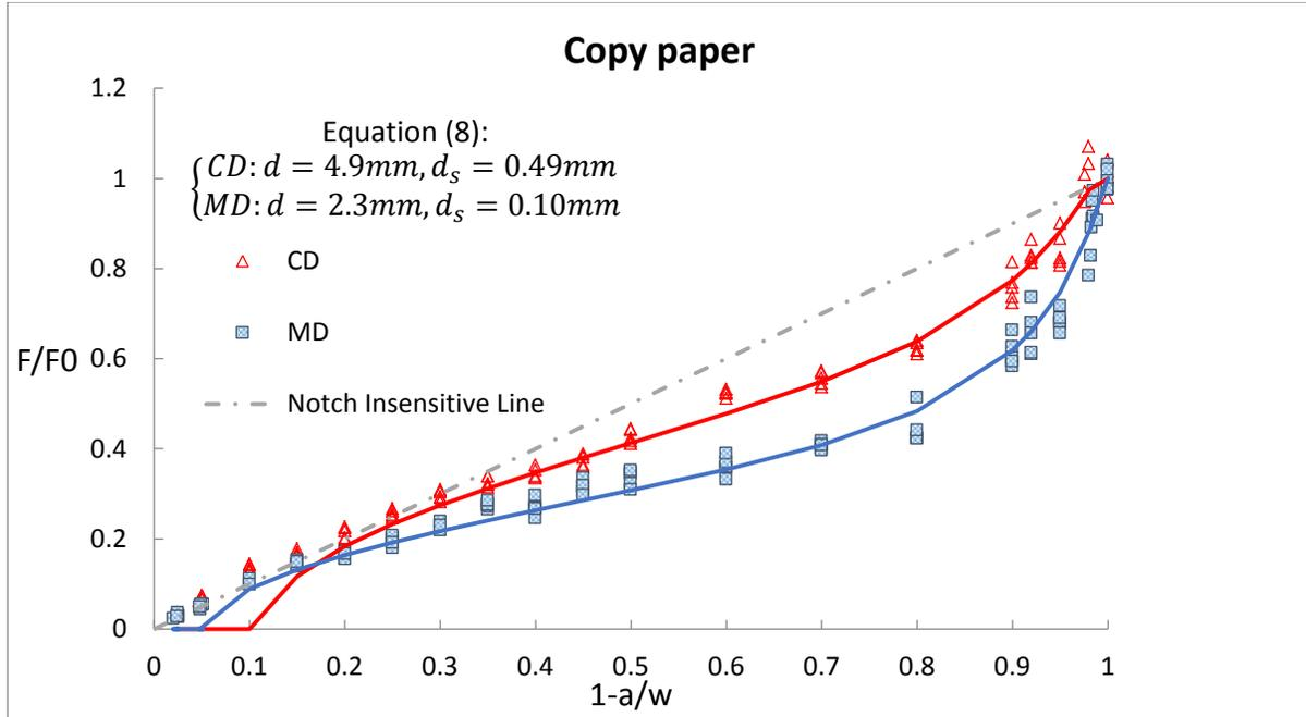
**Figure 4 DENT load ratio versus relative ligament length for Copy paper. The solid lines are the Equation (8) and the dash line is notch-insensitive line.**
