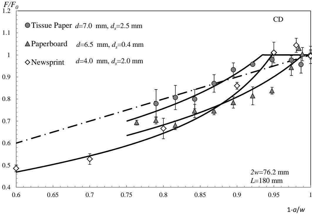
Figure 20. DENT results of load ratio versus relative ligament length for various papers in CD direction. Solid lines represent Equation (6). Dash-dot line represents notch-insensitive response  $F/F_0=1-a/w$ .
