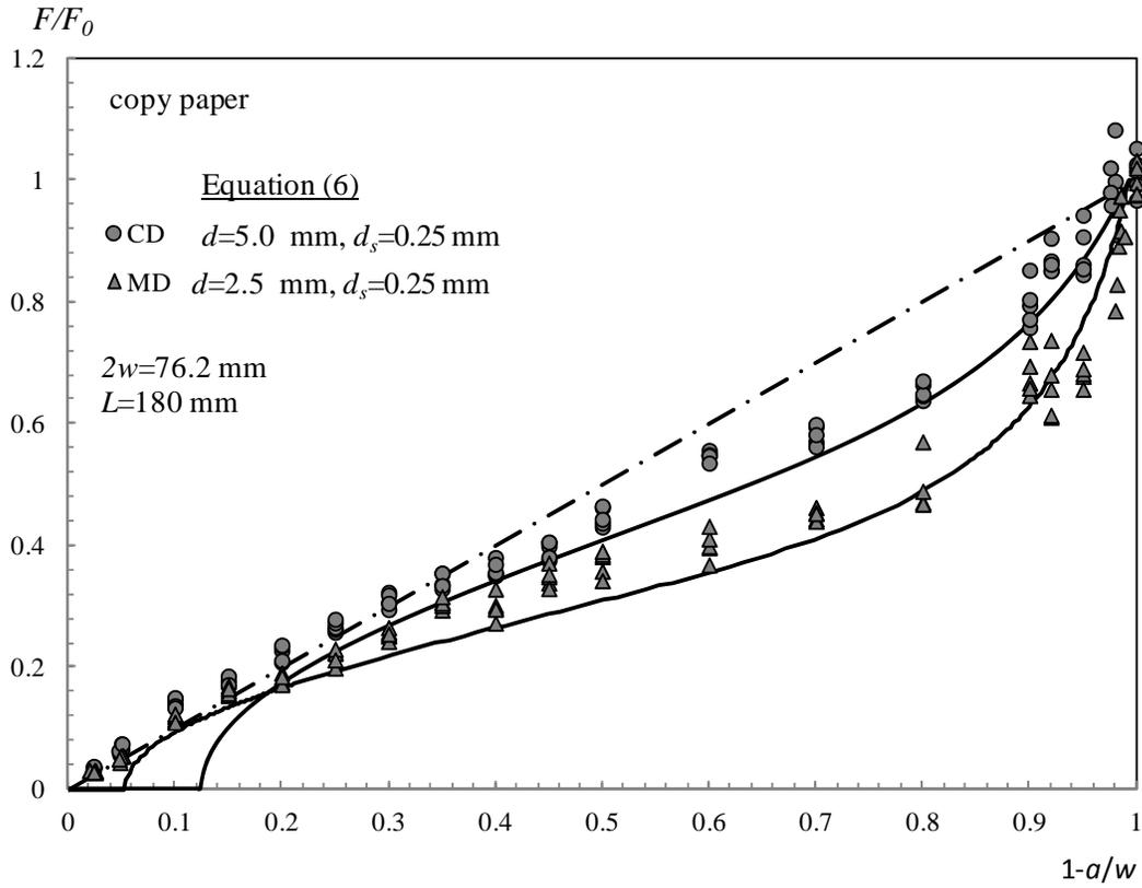
Figure 17. DENT results of load ratio versus relative ligament length for copy paper. Solid lines represent Equation (6). Dash-dot line represents notch-insensitive response  $F/F_0=1-a/w$ .
