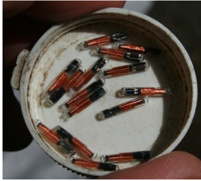
Figure 11 PIT tags used in the mark and recapture of Brook Trout. [photo by. JCWilliams]
