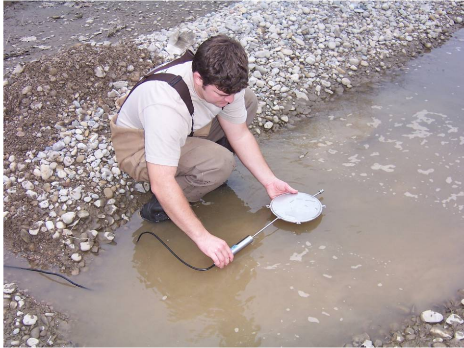
Figure 5. Placement of the vibrating-wire load-cell pressure sensor in a trench in the riverbed
