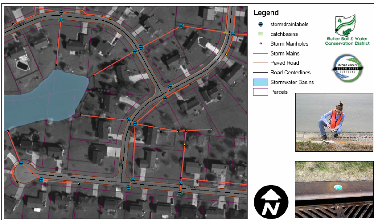
Figure 13. Storm Drain Labels Mapped in Butler County GIS System
