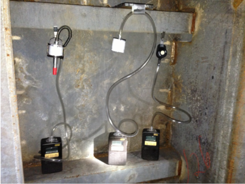
Figure 3-6: Photograph of Cyclone (left), Total (middle), and IOM Dual Sampler Arranged for Sampling
