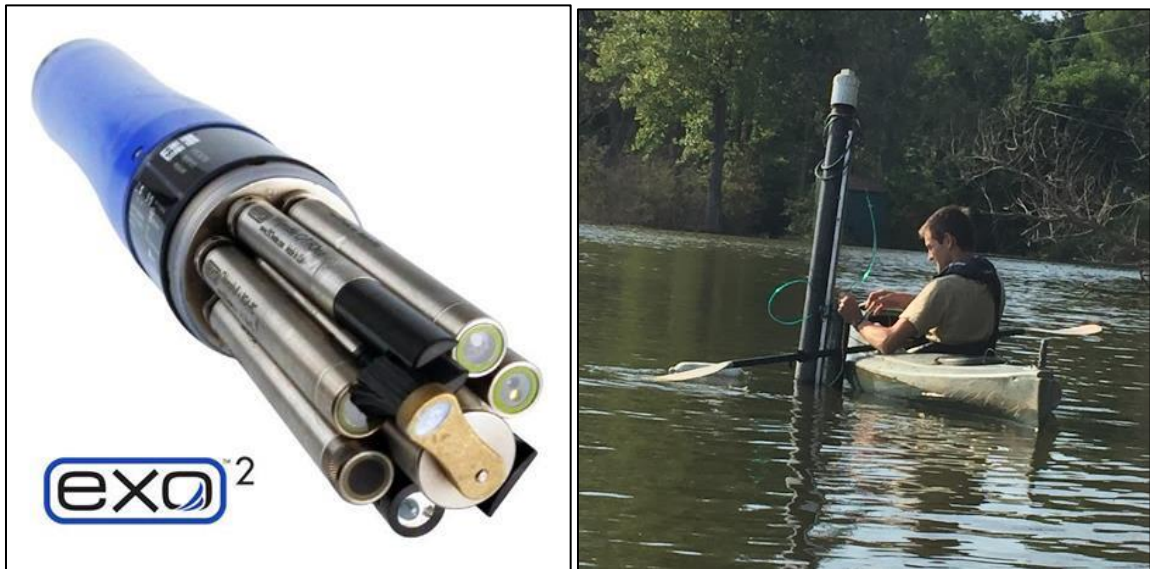
Figure 1) Pictured on the left is an EXO-2 sonde with various sensor probes attached at the bottom. On the right is a picture of EXO-2 field deployment at Old Woman Creek NERR. The EXO-2 is attached to an established pole with a vertical track for easy deployment and maintenance access.
