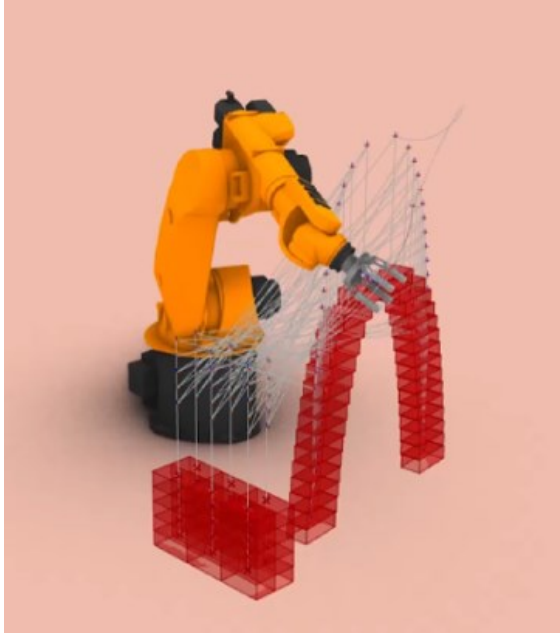
Figure 21: Kuka-Prc Model for Masonry Arch Construction
