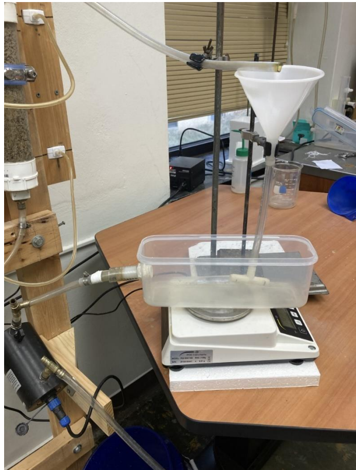
Figure 11. Mass Balance capable of continuous data output at a rate of 1 Hertz that is displayed via graphing accumulated mass of sediment lost due to piping failure.
