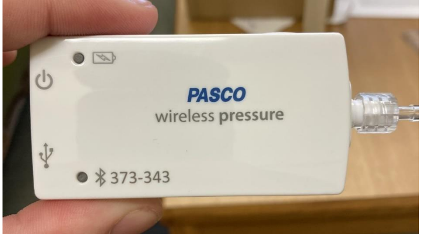
Figure 10. Pasco Pressure Sensor with Bluetooth capabilities containing a range of 0-400 Kilopascals (kPa) along with a capture collection rate maximum of 1000 Hertz (Hz)
