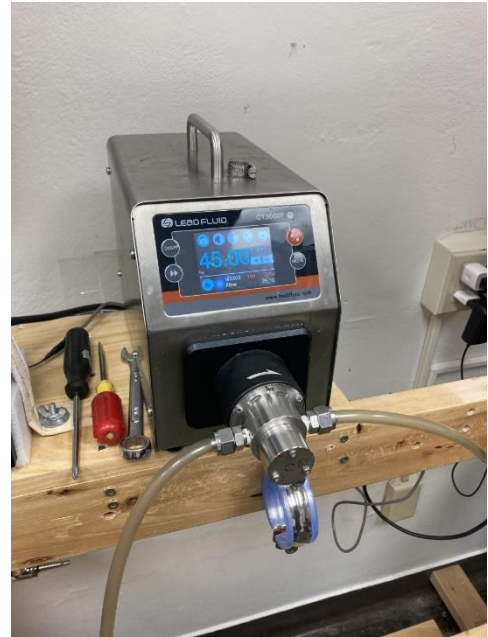
Figure 8. Leadfluid Gear Pump used for experimentation that allowed for a constant, controlled flow rate.
