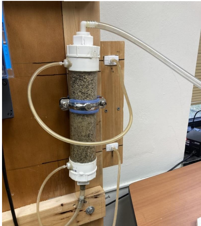
Figure 9. Sediment Column allowing for upward seepage flow. The column contains a filter with an aperture of 0.595mm on the bottom to prevent sediment returning into the tubing. No filter is present at the top of the column to allow for piping to occur.
