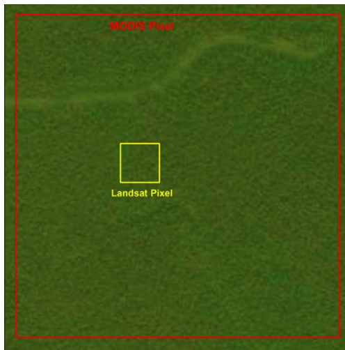
Figure 6: Extent of a MODIS pixel (250X250) and Landsat pixel (30X30) in Sundarbans area. Red box shows the boundary of the MODIS pixel and yellow box shows the boundary of the Landsat pixel (Source: ESRI Base Map).
