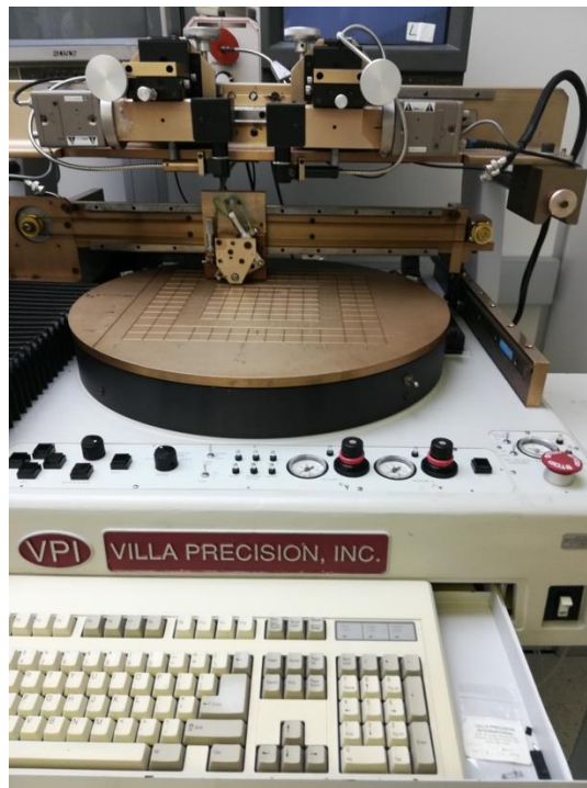
Figure B.1 Villa Precision, Inc (VPI-GS210) automated glass scriber machine
