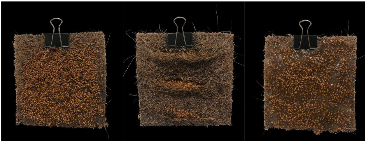
Figure 3.4: Envelor samples with straight seed (left), pocket (center), and Konjac Gum (right) treatments
