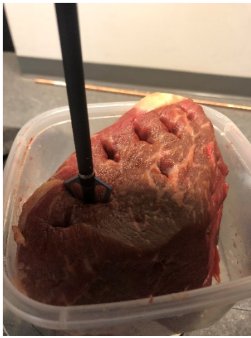
Figure 6: Penetration of field tip into the meat during the pilot study. Note the lack of stability in the matrix and the tenderizing effect of the continuous testing.
