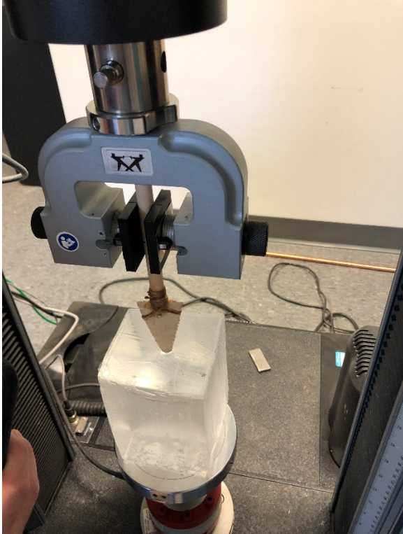
Figure 3: Manufactured stone tip penetrating ballistics gelatin during the pilot project.
