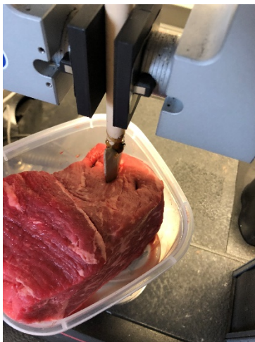
Figure 6: Penetration of field tip into the meat during the pilot study. Note the lack of stability in the matrix and the tenderizing effect of the continuous testing.
