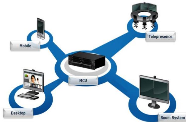
Figure 1.2 The MCU connecting multiple endpoints[27]
