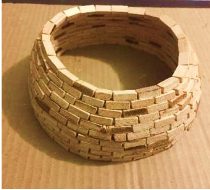
Figure 2.18: Small-scale model of a dome made to understand the construction technique
