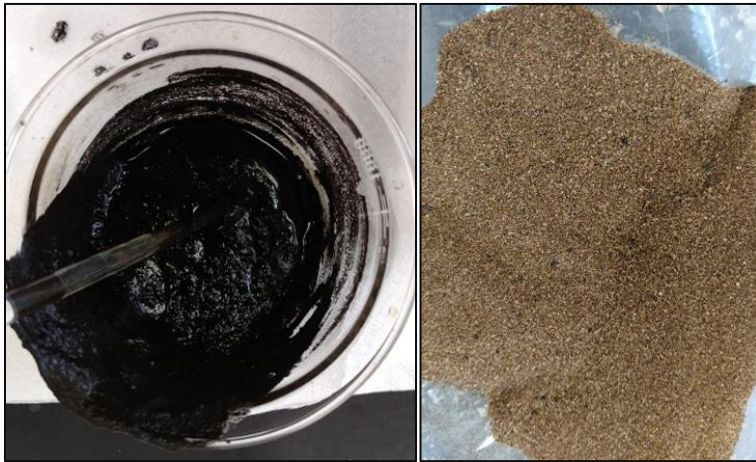
Figure 3. Left: Manganese oxide slurry generated by mixing potassium permanganate, sodium lactate, sand, and deionized water. Right: Mn-oxide coated sand rinsed with deionized water.
