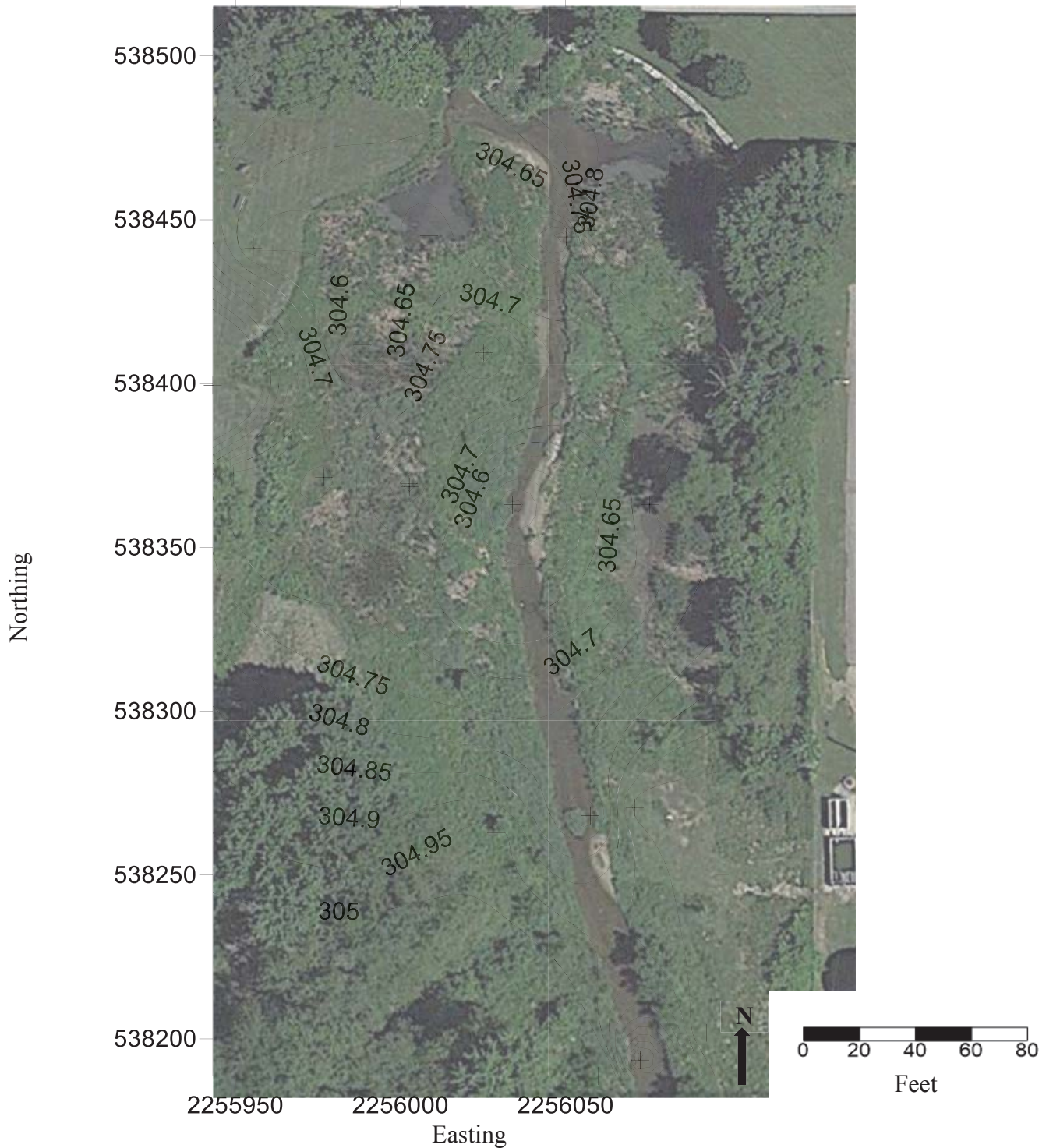
Figure 3.16. Topographic map created in Surfer using Ohio state plane coordinate system in feet with contour interval of 0.05 meters. Note: Kelsey Creek reach is referenced in the background and the black crosses represent well and piezometer locations.
