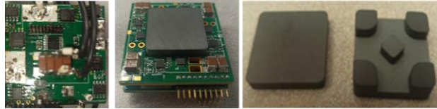
Figure 4-7 Prototype of the MASC and the core of the matrix autotransformer.
