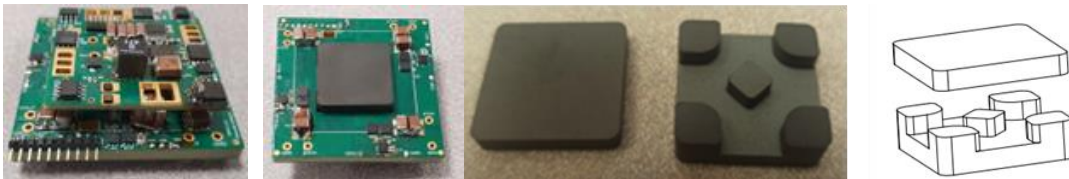
Figure 6-9 The prototype and the magnetic core
