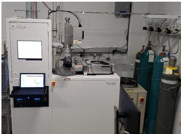
Figure 3.3: Veeco Fiji G2 Plasma-Enhance ALD used for deposition.
