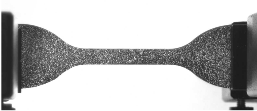
Figure 3.7: High-contrast speckle pattern applied to a tension specimen
